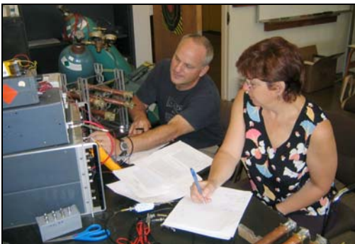
Professor of Physics Jim Alexander and high school physics teacher Deborah Lynn work together to monitor and adjust the voltage of the drift tube assembly they designed.
