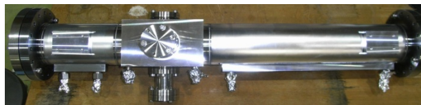
Figure 1: 0.9m long DLC coated Al Chamber after the surface roughing.
