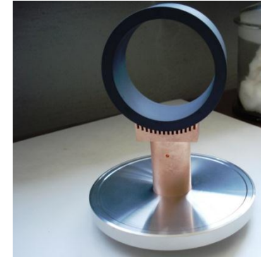
Absorbing ceramic ring brazed to the Cu stub
