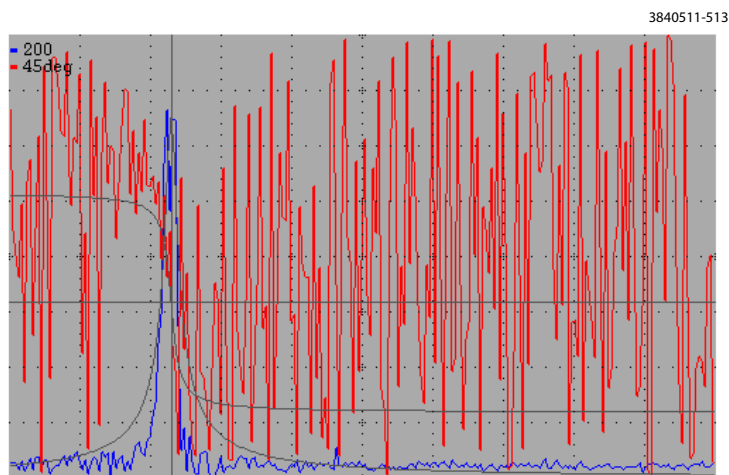
Figure 2.113: Frequency sweep over 10kHz. Blue trace is amplitude and red trace is phase error, showing fit to Lorentzian resonance model.
