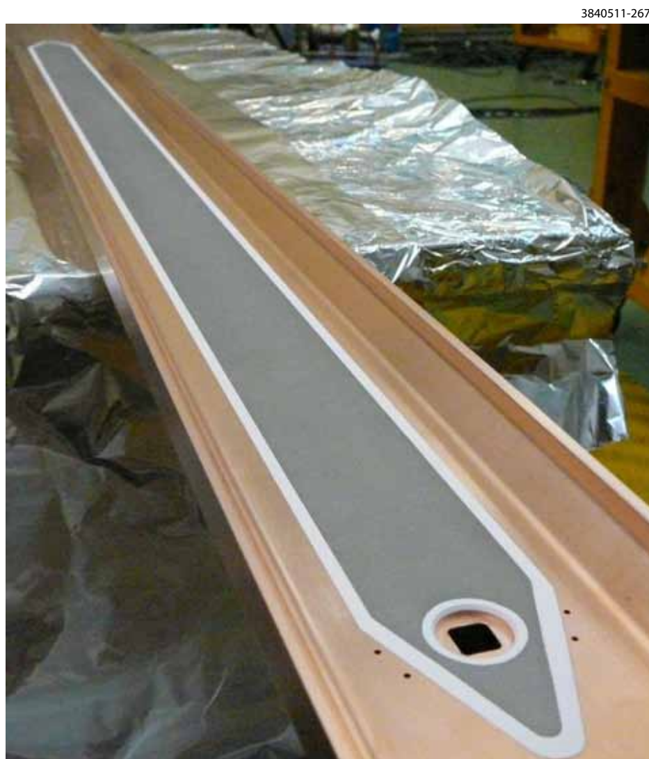
Figure 2.58: Photo of deposited electrode on the bottom of the SCW beam pipe.
