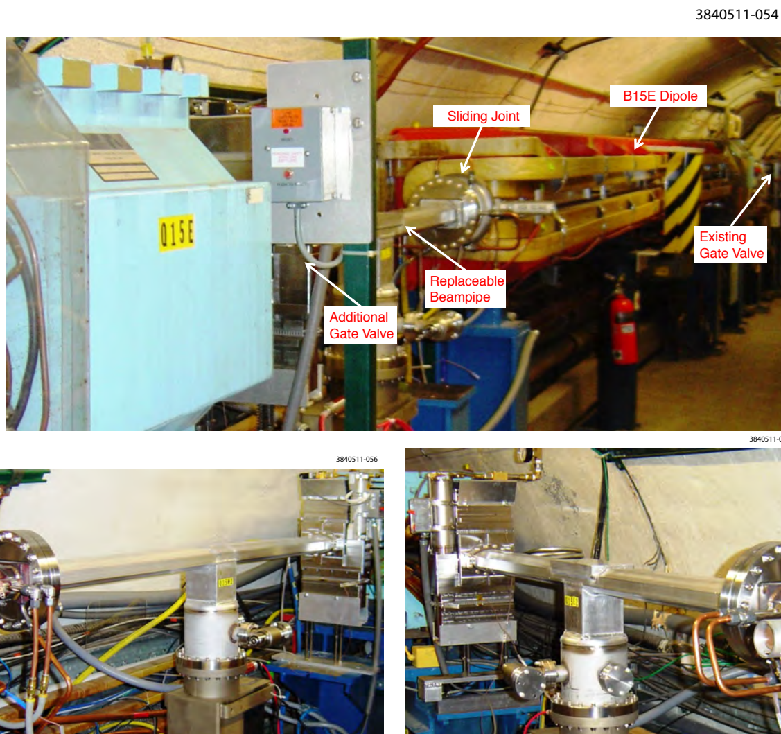
Figure 2.9: Two very short EC experimental sections were created in the CESR arcs. Top: photograph showing the chamber adjacent to Q15E, including the downstream bending magnet. Bottom: close-up photographs of the place-holder test chambers in Q15W (left) and Q15E (right).
