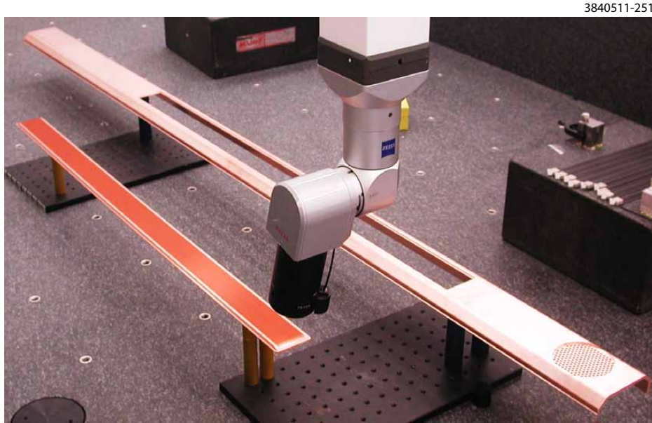
Figure 2.51: Bottom half of an SCW beam pipe with a cut-out and the groove plate during inspection on a CMM (Photo courtesy of Dawn Munson of LBNL)
