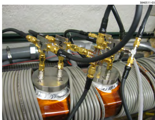
Figure 2.84: Photo of Shielded Pickups installed at 15E with the installed solenoid winding
