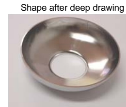
Deep drawing by one flexible tool
