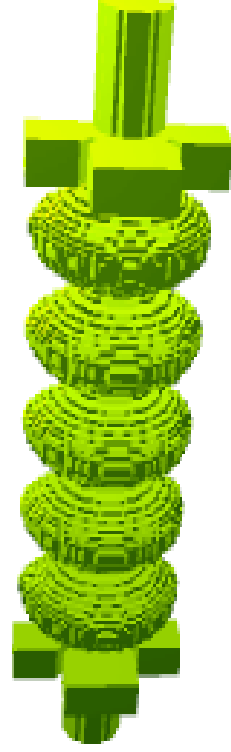
5-cell cavity with waveguide loads.
