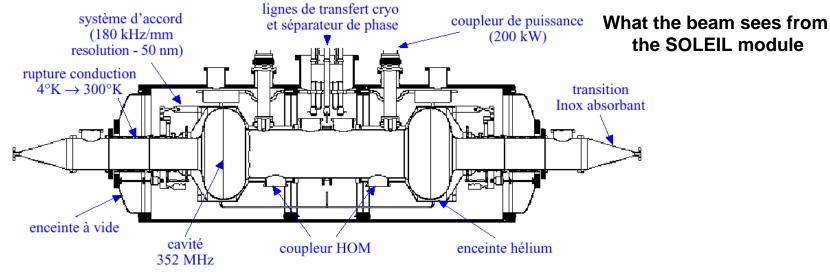
Two single cell cavities (352 MHz) in one vacuum vessel
