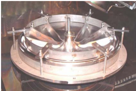
ANL 3-Spoke resonator end-plate with self-compensating design for minimum df/dP
