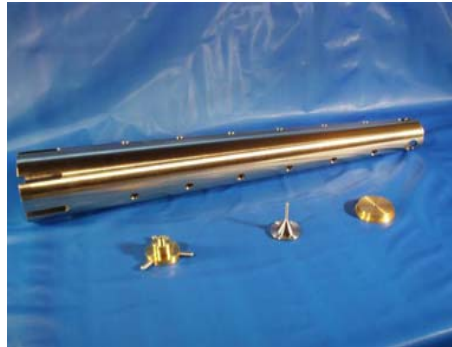
4-gap, 48 MHz QWR with vibration damper
