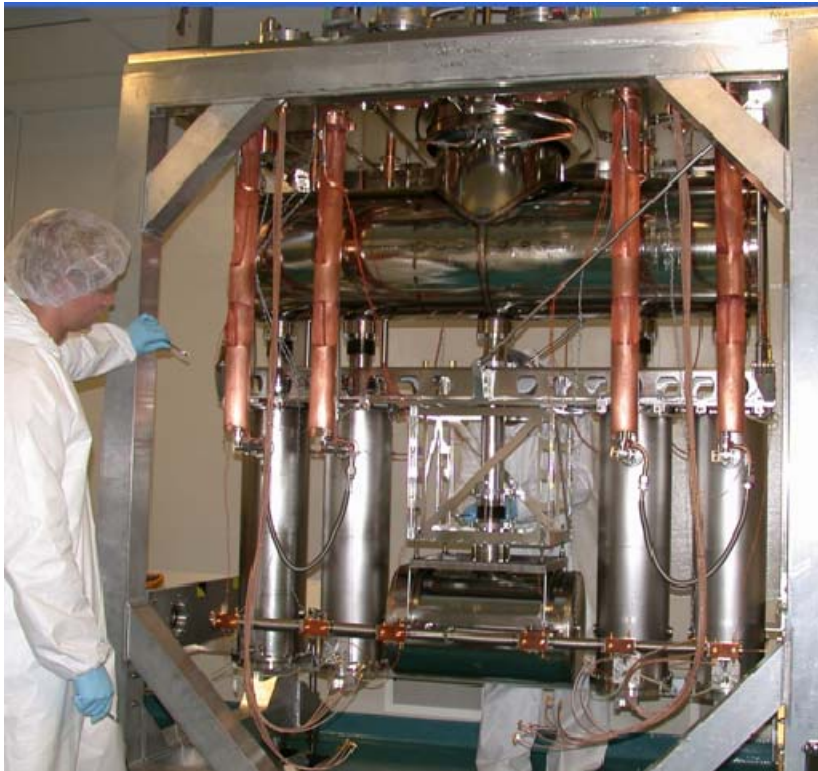
Common vacuum cryostat (TRIUMF)
