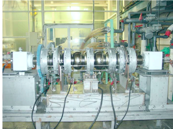
Electropolishing @Nomura Plating on May 27
