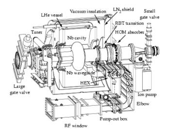
FIG. 1: SRF cryomodule and its components
