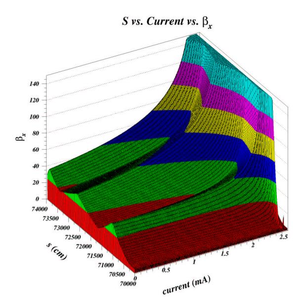
FIG. 12: Plot of the change in the  $\beta_x$  function around the entire ring as a function of the current in each beam bunch of the second beam. Note the spike at current  $\approx 2.5$  mA.
