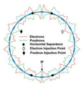
FIG. 3: Conceptual diagram of pretzel orbit in the CESR ring, along with the placements of separators and particle injection points.
