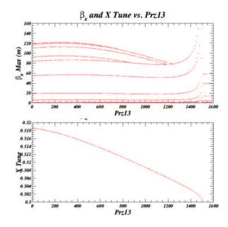
FIG. 15: The top graph again is a side view of Fig. 14 showing the spikes in the  $\beta_x$  function. The lower graph is a plot of the x tune value during the same run. The spike again corresponds to the point at which the x tune reaches the half integer resonance.
