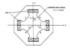
FIG. 2: Cross section of a quadrupole magnet
