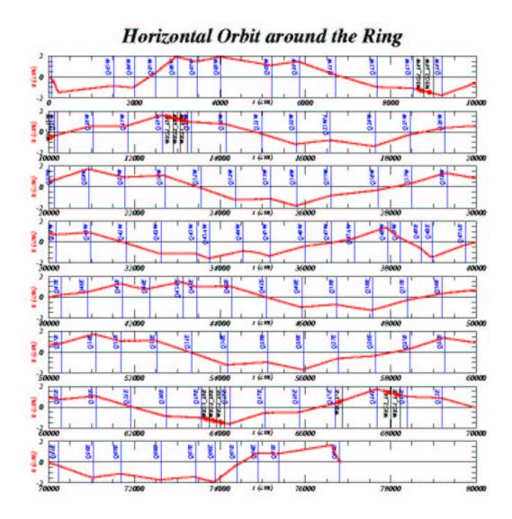
FIG. 5: Plot of the x orbit traced through one revolution around the ring, with all quadrupole and wiggler magnets labeled. The zero line represents the theoretical orbit at the center of the beampipe.
