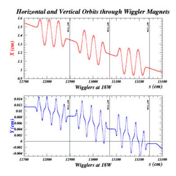
FIG. 7: Plot of the x and y orbits as they pass through the 3 wiggler magnets at position 18W.
