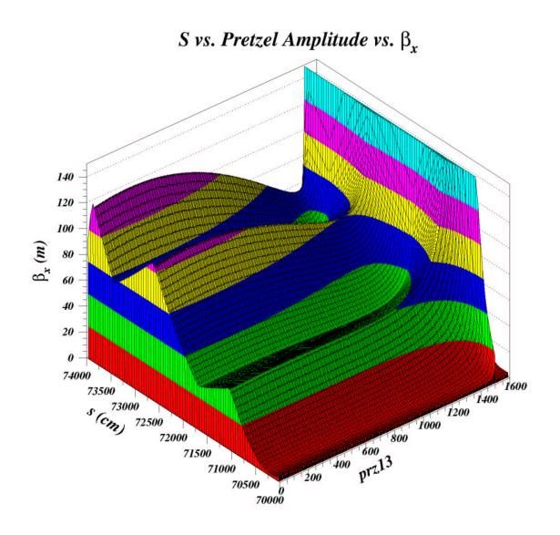
FIG. 14: Plot of the change in the  $\beta_x$  function around the entire as a function of the amplitude of the pretzel orbit. Note the spike at prz13  $\approx 1500$ .
