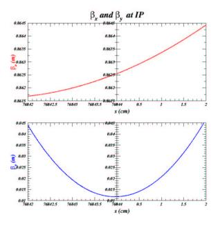
FIG. 11: Close up view of the x and y orbits and the  $\beta_x$  and  $\beta_y$  functions as they cross the IP.
