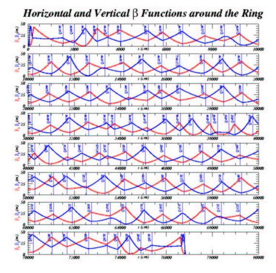
FIG. 8: Plot of  $\beta_x$  and  $\beta_y$  traced through one revolution around the ring, with all quadrupole magnets labeled.
