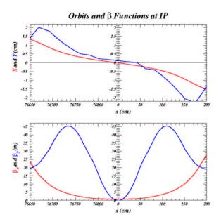
FIG. 10: Plot of the x and y orbits and the  $\beta_x$  and  $\beta_y$  functions as they cross the IP.
