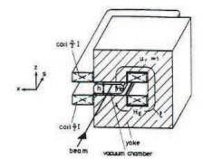
FIG. 1: Cross section of a dipole magnet
