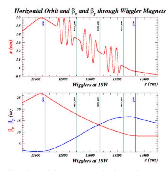
FIG. 9: Plots of the x,  $\beta_x$  and  $\beta_y$  functions as they pass through the 3 wiggler magnets at position 18W.
