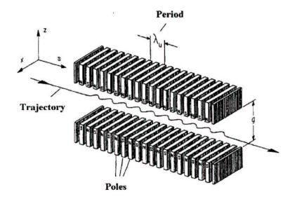
FIG. 4: Diagram of a CHESS wiggler magnet
