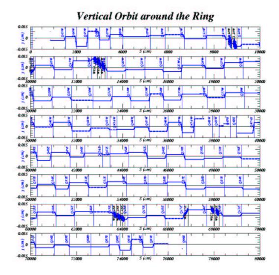
FIG. 6: Plot of the y orbit traced through one revolution around the ring, with all quadrupole and wiggler magnets labeled. The zero line represents the theoretical orbit at the center of the beampipe.
