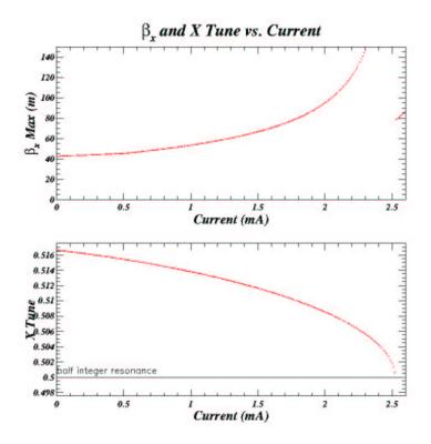
FIG. 13: The top graph is a side view of Fig. 12 showing the spikes in the  $\beta_x$  function. The lower graph is a plot of the x tune value during the same run. The spike corresponds to the point at which the x tune reaches the half integer resonance.
