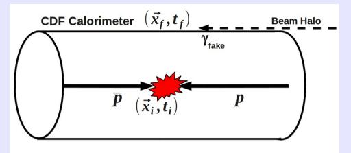
Beam halo particles are typically muons produced beam interactions upstream of the detector
