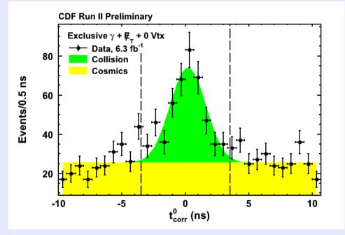
Good Vertex: Right-Vertex Events =  $880 \pm 70$ Wrong-Vertex Events =  $670 \pm 80$ Cosmics Rate =  $31.9 \pm 0.7$  No Vertex: Collision Events =  $250 \pm 30$ Collision Mean =  $0.2 \pm 0.1$ Cosmics Rate =  $38.1 \pm 0.8$
