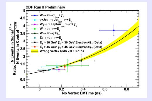
We isolate no vertex events in Monte Carlo and electron data and fit to find the no vertex mean.
