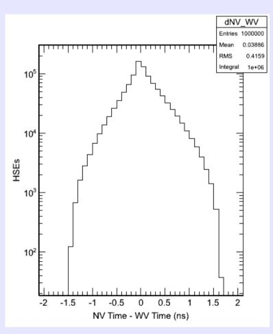
Wrong vertices are distributed according the the beam profile. In Z, they are Gaussian distributed with a mean of ~0 cm and an RMS of ~ 28 cm. In T, they are Gaussian distributed with a mean of ~0 ns and an RMS ~1.28 ns.
