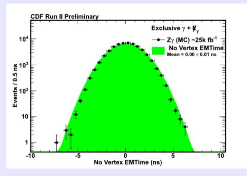
If no good vertex reconstructed, we can still construct the raw time variable: the corrected time, around a vertex with Z = 0 and T = 0.
