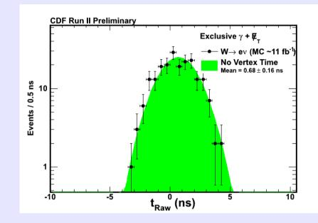
The means for wrong-vertex events and no-vertex events are very close. The smearings due to the distribution of vertices only smooth out any non-Gaussian behavior.
