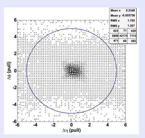
Vetoing reconstructed photons with a track with  $\Delta R(pull) < 5$  removes 73% of fake photons while accepting 95% of real photons.
