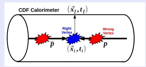
The wrong vertex distribution has an RMS ~ 2.0 ns, mostly due to the time profile of the beam spot.
