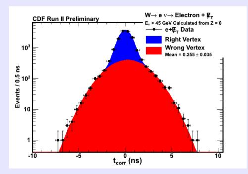
If we cut on  $E_{\tau}$  calculated relative to Z = 0, we limit how wrong we can be. The measured time and  $E_{\tau}$  are no longer completely coupled, and the mean shift is halved!
