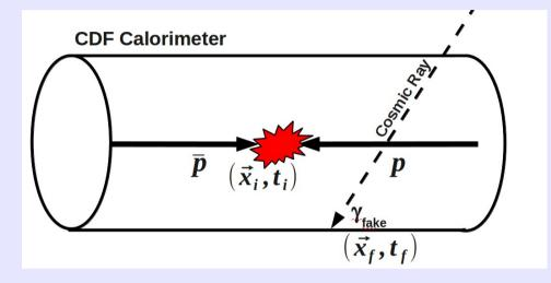
This is uncorrelated with the bunch structure of the beam, so the rate of recording such events is flat in time, except near the opening and closing of the energy integration window Cosmic rays occasionally reach the detector and leave an energy deposit which is reconstructed as a photon
