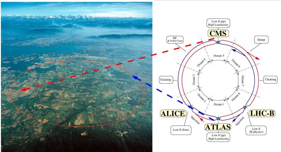
Proton-proton collider at CERN in Geneva, Switzerland2011 operation: collisions at 7 TeV center of mass energy2 general purpose experiments: ATLAS and CMS
