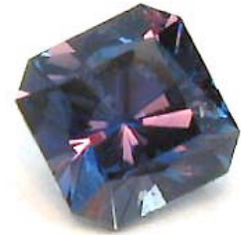
Sapphire Melting point: 2050°C
