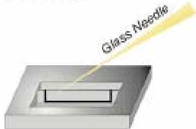
Pick up of TEM lamella with Lift-out Tool
