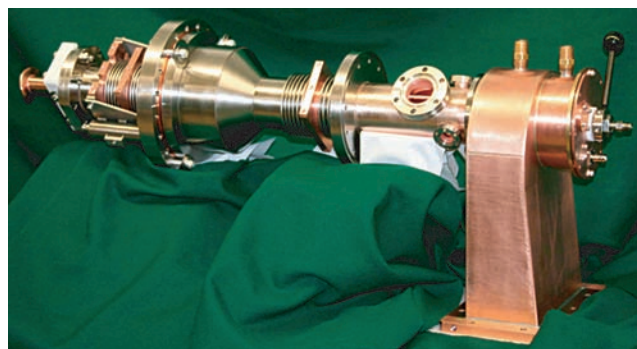
Figure 5: The prototype RF power coupler. 1.3 GHz microwave power enters the waveguide to coaxial coupler transition at the right-hand side, and is fed to the RF cavity at the end of the coaxial line on the far left-hand side. Of the three flanges along the coaxial section, the left-hand one is at 2 K, the central (largest) one is at 80 K, and the right-hand one is at room temperature. Thin copper plating inside the several bellows, and thermal intercepts serve to limit the power deposited at cryogenic temperatures.
