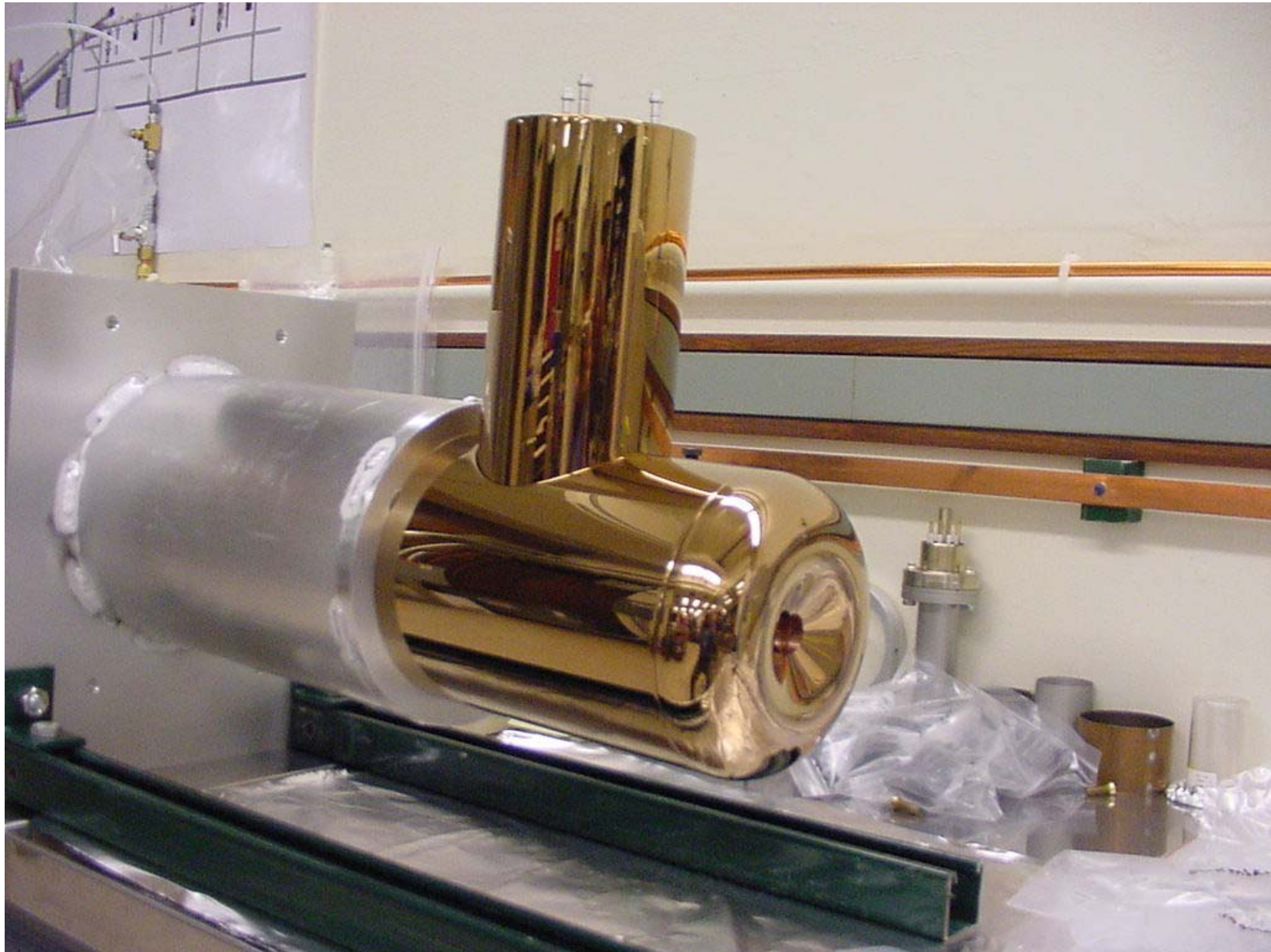
Cathode electrode structure during assembly
