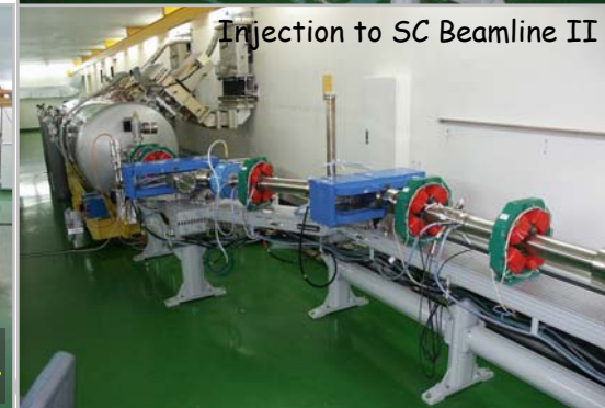
Two 4-cell cavities 352 MHz/~15 MeV
