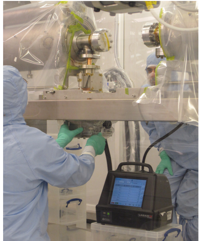
Figure 5: Cold coupler insertion into the cavity port in the ISO4 cleanroom.
