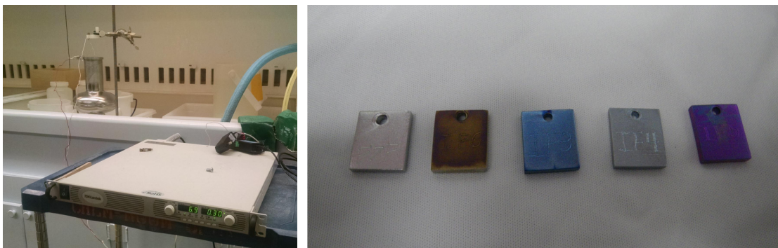
Figure 5.10: Left, the chemistry setup for anodising the interior of a niobium cavity. Right, a series of samples with different voltages of pre-anodisation, these being (from L to R): 0 (none), 5, 15, 30, and 60 volts.
