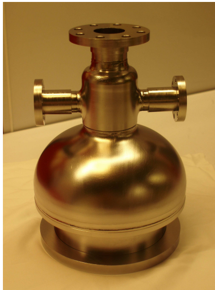
Figure 3.26: Finished TE mushroom cavity after a heavy BCP.
