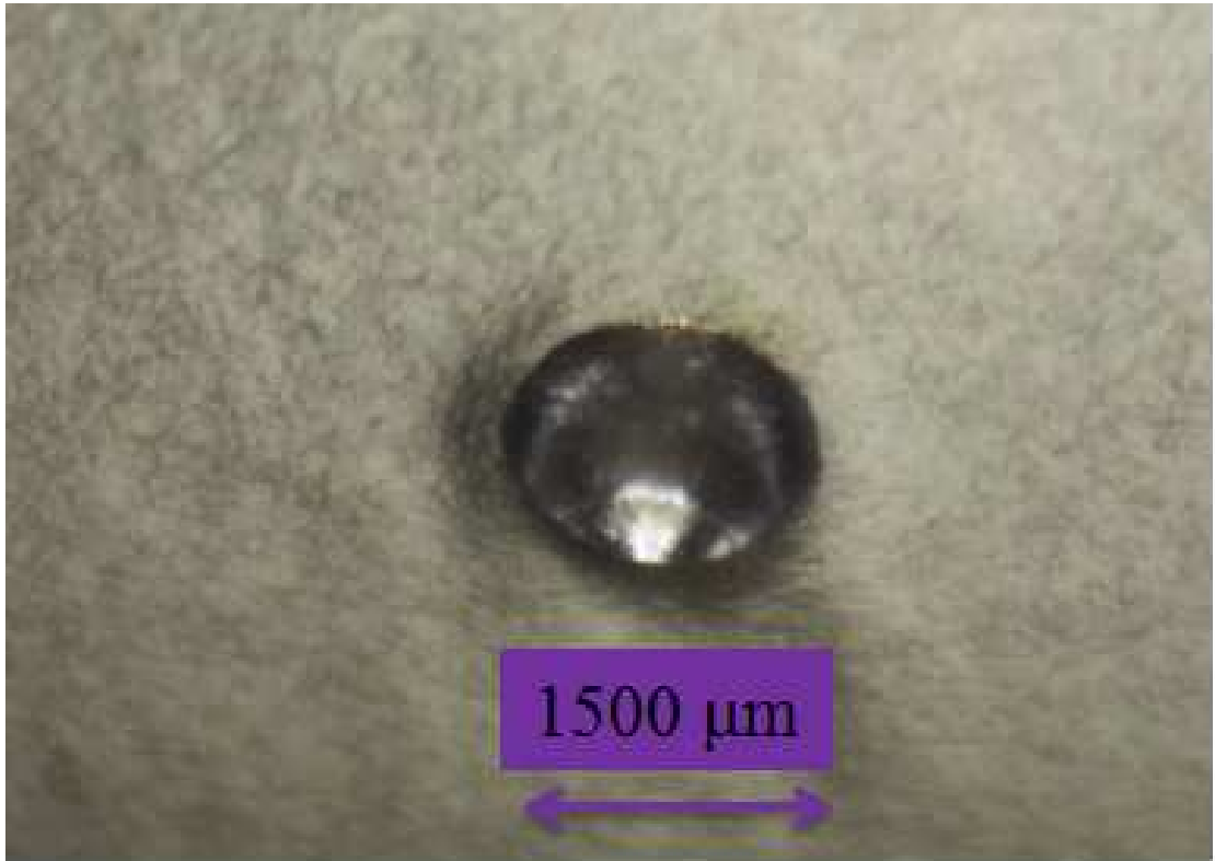
Figure 5.12: Optical inspection image of pit #30.
