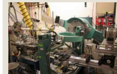
The Huber 6-circle diffractometer used for conducting crystallographic and diffraction studies at CHESS.
