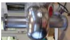
New cavity shape developed by LEPP to reach 50 million volts per meter.
