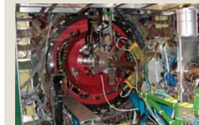
CLEO is a high-energy physics instrument that detects, measures and analyzes electron-positron collision events.
