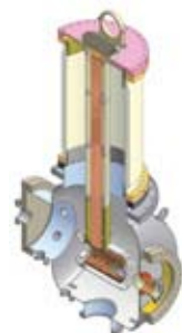
This photocathode gun, which is part of the ERL injector, is where the electrons are created.
