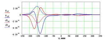
Figure 7: Normalized transverse fields on the axis of the injector cavity for a relative penetration depth error of 1 mm. The coordinate z = 0 corresponds to the cavity center.  $E_{y1}$ ,  $B_{x1}$  and  $E_{y2}$ ,  $B_{x2}$  were calculated respectively for shorted and open coupler.
