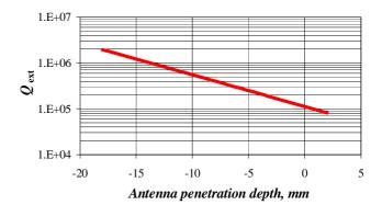
Figure 2: Dependence of  $Q_{\rm ext}$  of a single coupler on the penetration of the antenna tip into the cavity beam pipe. The  $Q_{\rm ext}$  of a twin coupler is twice as low.
