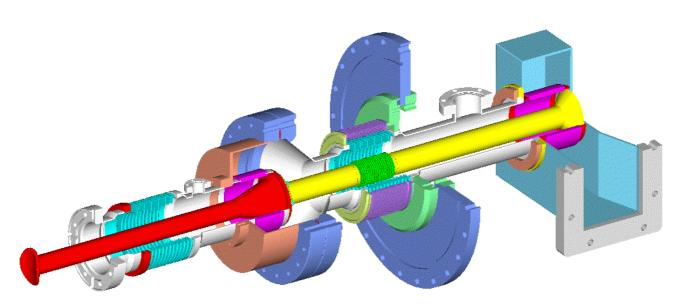
Figure 3: 3D view of the injector cavity coupler.
