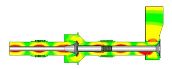
Figure 5: Electric fields in the coupler.
