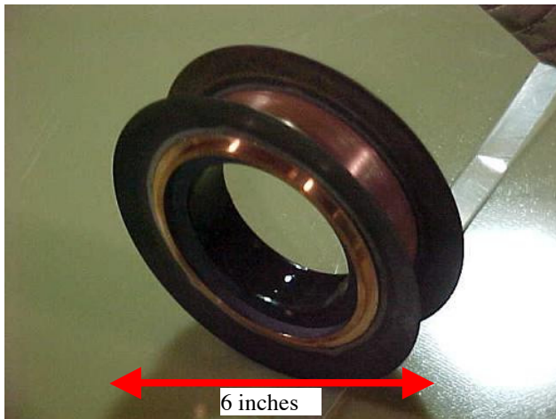
Figure 4: Glass coated ferrite in the final sub assembly module
