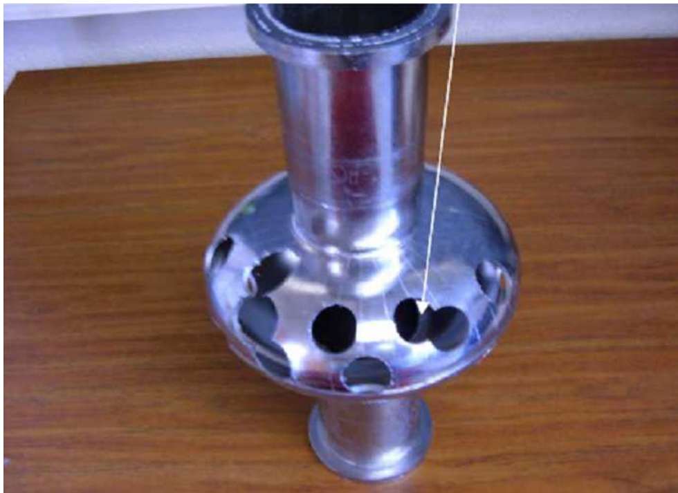
Figure 6.2: The picture of the cavity, which had hot and cold areas cut out for analysis. Arrow indicates one of the samples.
