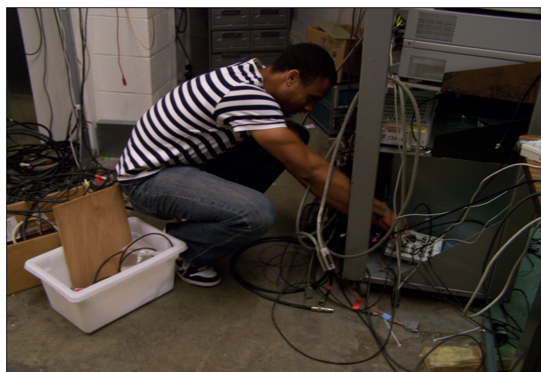
Connecting the Helium level monitor to the data acquisition card (daq card)
