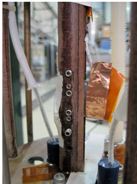
Figure 8: Experimental Setup of the Old System. In the old system, the low resistance of superconducting materials was used to find the sample's critical temperature, rather than their ability to expel all magnetic flux.
