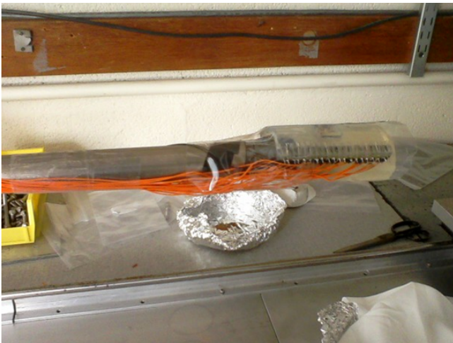
Figure 3: The actual light/mirror portion of the light/mirror apparatus. The mirror is located beneath a slit in the gel substance. This substance spreads out the light from the LEDs reducing glare on the cavity surface.
