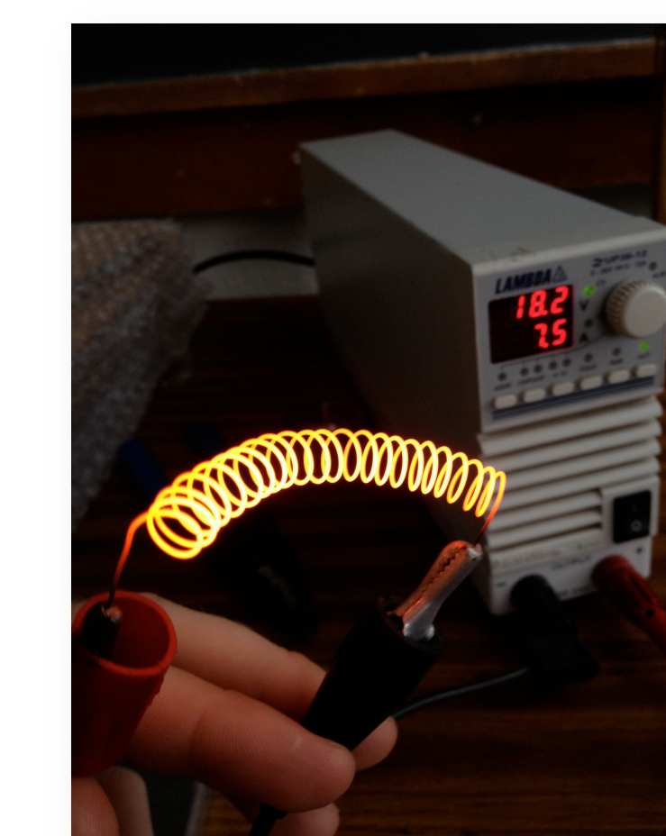
Heater coil test
