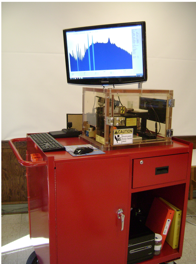
FIG. 1: The entire XRF cart. The X-ray source, sample, and detector are all contained in the lead acrylic enclosure on top of the cart. The digital pulse processor and a computer are also located in the cart; collected spectra are displayed on the monitor.
