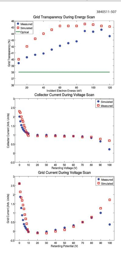
Figure 2.72: Plots showing electron gun studies of the performance of the thin RFA structure with a front plate with holes matching the wiggler vacuum chamber specifications. The top plot shows the fraction of electrons reaching the collector versus the energy of the incident electrons. The bottom pair of plots show the collector and grid currents observed during a retarding voltage scan with 110 eV incident electrons.
