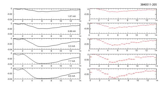
Figure 5.82: Comparison of measured single bunch signals for various electron bunch currents (left column) to the ECLOUD model (right column) after improving the modeled photoelectron energy distributions.
