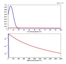
Figure 5.81: Low- and high-energy regions of the photoelectron energy distributions used to model the measured signals shown in Fig. 5.80. The original low-energy distribution shown in blue results in dramatic discrepancy with the signals observed in the case of an electron beam. The modified distribution shown in red provides good agreement with the observed signals.
