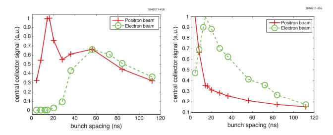
Figure 5.36: Central collector signal in a dipole RFA as a function of bunch spacing, for a 20 bunch train with 3.5 mA ( $5.6 \times 10^{10}$  particles) per bunch, at 5.3 GeV. Left: SLAC chicane RFA, right: CESR dipole RFA
