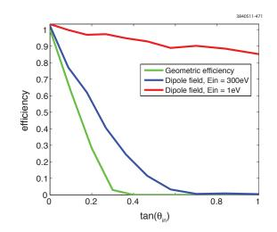
Figure 5.13: Simulated RFA efficiency vs incident angle for a CESR dipole RFA, with a 790 G magnetic field. This corresponds to operation at 2.1 GeV.
