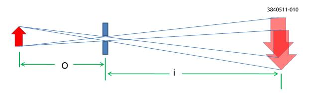
Figure 2.99: Schematic showing the convoluted image in pinhole focusing.
