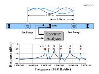
Figure 5.56: Sketch of 43E at CESRTA, where a BPM Detector is located between two ion pumps with longitudinal slots. The measured resonances follow the expected  $f^2 = f_c^2 + \left(\frac{nc}{2L}\right)^2$  of a rectangular cavity.
