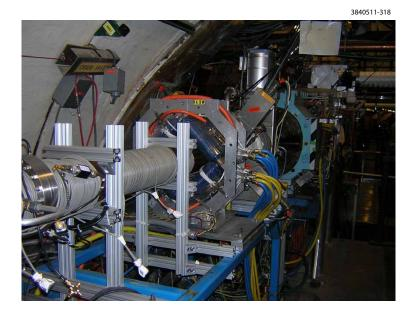
Figure 2.131: View of solenoidal field windings on the L3 straight section vacuum chambers.
