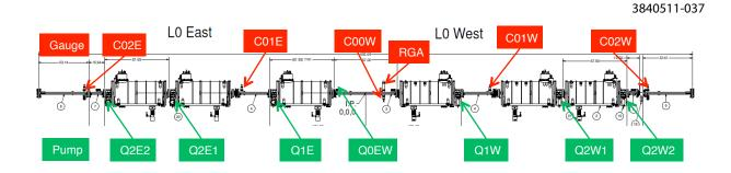
Figure 2.3: Vacuum Pumping and Instrumentation in the L0 Center CESRTA EC experimental region. At locations (labeled in *GREEN* as Q2E2, Q2E1, Q1E, Q1W, Q2W1 and Q2W2), a combination of a NEG and a small SIP is installed, while at the center of the region (labeled in *GREEN* as Q0EW), a large SIP is installed. Five cold-cathode ion gauges and a residual gas analyzer (as labeled in *RED*) are also installed in the region to monitor the vacuum system performance.
