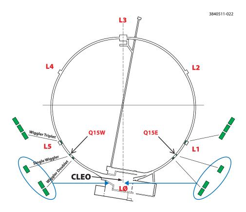
Figure 2.1: The reconfiguration of the CESR vacuum system provided space in two long regions in L0 and L3, and two flexible short regions at Q15W and Q15E. Hardware for electron cloud studies was installed in these regions.
