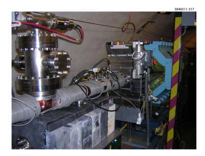
Figure 2.130: View of solenoid windings on a second typical arc vacuum chamber.
