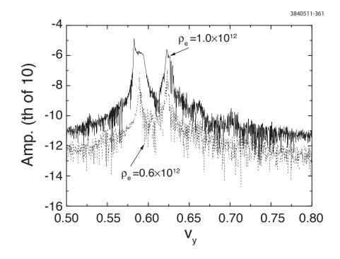
Figure 6.84: Frequency spectrum with feedback at 2 GeV. The electron cloud density  $\rho_e$  is in units of m<sup>-3</sup>.
