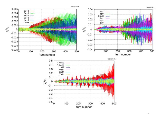
Figure 6.90: Motion of vertical bunch centroid for varying cloud densities, in units of  $m^{-3}$ .
