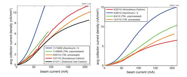
Figure 5.23: Comparison of different beam pipe coatings, 15E (left), and 15W (right) drift RFAs. Plots show average collector signal vs beam current for **20 bunches** of **electrons** with **14 ns** spacing, at beam energy **5.3 GeV**. Note that the aluminum chamber signals are divided by 3.
