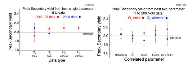
Figure 6.25: The best fit peak secondary emission yield parameter, as determined from a singleparameter fit, vs. data type (left); The best fit peak secondary emission yield parameter, as determined from a two-parameter fit, vs. the other parameter in the fit (right).
