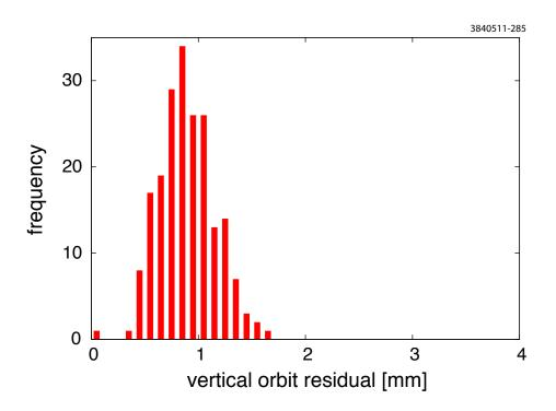
Figure 3.3: Distribution of residual vertical orbit offset for 200 configurations each generated with gaussian vertical quadrupole offsets with  $\sigma_y = 35 \,\mu\text{m}$  and bend rolls with  $\sigma_{\theta} = 152 \,\mu\text{m}$ .
