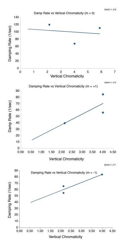
Figure 6.66: Single bunch damping rate vs. vertical chromaticity. Top: vertical dipole mode. Center: vertical m = +1 head-tail mode. Bottom: vertical m = -1 head-tail mode.
