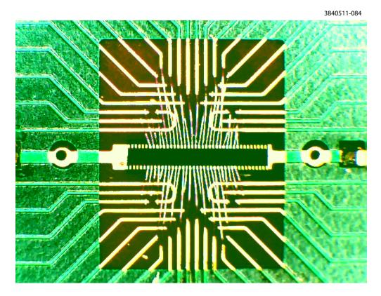
Figure 2.93: xBSM diode detector
