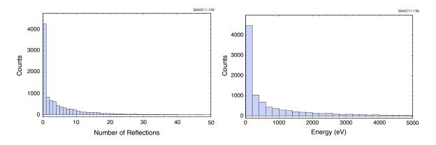
Figure 5.3: Reflection distribution (left) and energy distribution (right). The mean number of reflections is 5.1.
