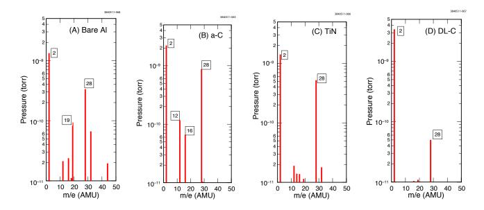
Figure 2.16: Typical RGA spectra for four Q15 EC test chambers with different surfaces, as labeled. All RGA spectra were recorded during CHESS operations, with  $\sim 400$  mA stored beam current in CESR, after significant beam processing (with the beam dose over 400 Amp·Hr).
