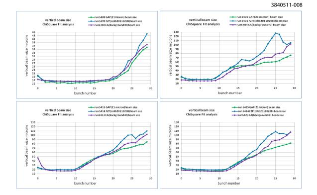
Figure 2.102: Beam size measurements with three optics elements, in four running conditions: (a) tuned for small beam size with 0.50ma/bunch, (b) same, 0.75 ma/bunch, (c) high chromaticity, (d) high chromaticity with precursor bunch 182ns before train.
