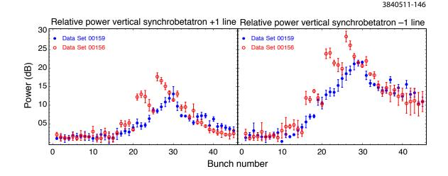
Figure 6.52: Data sets 156 and 159: vertical head-tail lines compared. Both sets have 45 bunches, the same chromaticity [ (H,V) = (1.34, 1.99) ] and bunch current (0.74 mA), but different values of the single-bunch vertical emittance, as follows: 156, Vertical emittance ~ 20 pm; 159, Vertical emittance ~ 300 pm
