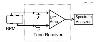
Figure 2.110: Simple block diagram of a narrow-band tune receiver, shown in the mode where it can detect both the horizontal and vertical betatron tunes.
