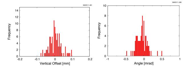
Figure 3.1: (Left) Distribution of measured vertical offsets of ring quadrupoles. The root mean square of the distribution is 35  $\mu$ m. (Right) Distribution of measured rolls of ring dipoles.  $\sigma_{\theta} = 152 \ \mu$ -rad.
