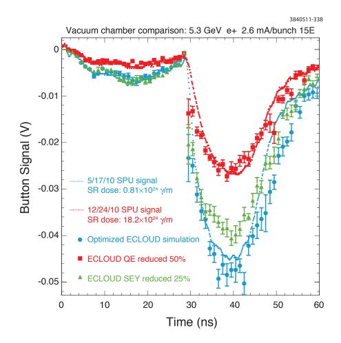
Figure 5.91: Shielded pickup signals measured in an a-C-coated chamber in May (blue dotted line) and December (red dotted line) of 2010 for two 5.3 GeV, 28-ns-spaced bunches each carrying  $4.8 \times 10^{10}$  positrons. The ECLOUD model optimized for the May data is shown as blue circles, the error bars showing the signal macroparticle statistical uncertainties.
