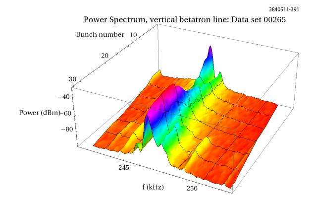
Figure 6.57: Data set 265: Bunch-by-bunch power spectrum: detail at vertical betatron line, 4 GeV. Chromaticity: (H,V) = (1.3, 1.4). Bunch current = 1.1 mA.
