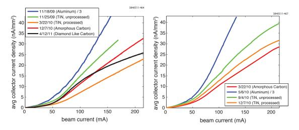
Figure 5.22: Comparison of different beam pipe coatings, 15E (left), and 15W (right) drift RFAs. Plots show average collector signal vs beam current for **20 bunches** of **positrons** with **14 ns** spacing, at beam energy **5.3 GeV**. Note that the aluminum chamber signals are divided by 3.
