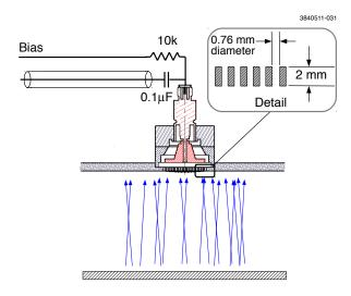
Figure 2.81: Shielded pickups are assembled in pairs. The longitudinal pair provide redundant measurement of the cloud along the beampipe centerline.
