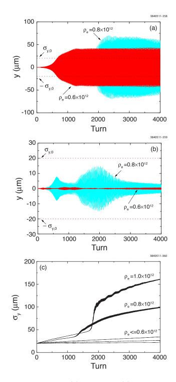
Figure 6.83: Evolution of the dipole motion (a) without and (b) with feedback at 2 GeV. (c) Vertical beam size growth with feedback at 2 GeV. The electron cloud density  $\rho_e$  is in units of m<sup>-3</sup>.
