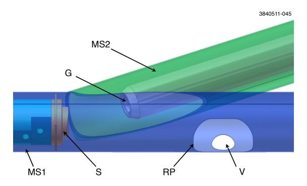
Figure 2.87: Magnetic shielding for SEY system. The sample (S) is inside Magnetic Shield 1 (MS1). The electron gun (G) is inside Magnetic Shield 2 (MS2). Magnetic Shield 1 has a Sample Replacement Port (RP; the patch is not shown) and a hole at the pumping port for vacuum pumping (V).
