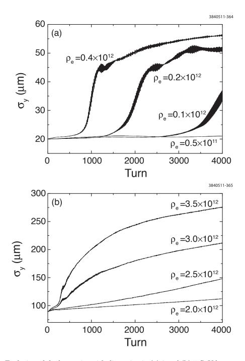
Figure 6.86: Evolution of the beam size with dispersion in (a) 2 and (b) 5 GeV beam energies. The ecloud density  $\rho_e$  is in units of m<sup>-3</sup>.
