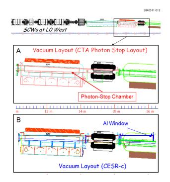
Figure 2.6: A specially designed photon-stop chamber (A) replaced CESR-c era FLM chambers (B), enabling operations of L0 SCWs with a positron beam at 5 GeV.
