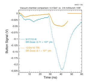
Figure 5.94: SPU signals exhibiting the difference in cloud buildup characteristics between a TiN-coated aluminum chamber and an uncoated aluminum chamber with a factor of ten lower synchrotron radiation dose.
