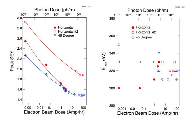
Figure 5.49: Dependence of SEY peak (left) and  $E_{\text{max}}$  (right) on dose for Al6061-T6 samples in the horizontal and  $45^{\circ}$  stations.
