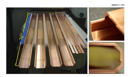
Figure 2.46: The copper beam pipes are split into two halves with EB-weld preps ready for cleaning and EB-welding. (Photos: courtesy of Dawn Munson of LBNL)
