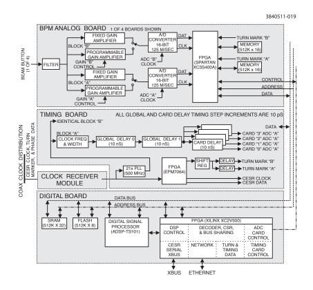
Figure 2.90: BPM module functional diagram
