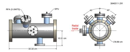
Figure 2.27: EC Diagnostic chamber with NEG thin film coating.
