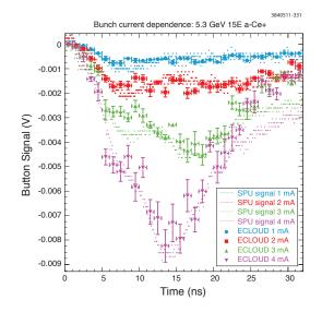
Figure 5.83: Modeled and measured leading SPU signals for bunch currents of 1, 2, 3 and 4 mA/bunch. The dramatically varying amplitudes and shapes are successfully reproduced by tuning the modeled photoelectron energy distribution as described in the text.
