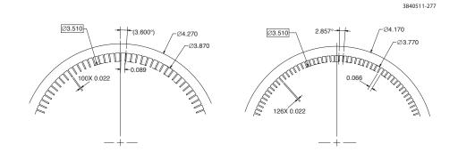
Figure 2.21: Details of rectangular grooves of two different groove depths on PEP-II aluminum beam pipes. The left shows grooves with depth of 4.5 mm, and right with depth of 3.3 mm. The beam pipes were extruded with type 6063-T6 aluminum alloy.
