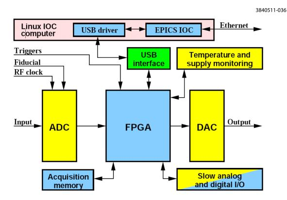
Figure 2.116: System overview of the Dimtel iGp 4 ns signal processor.
