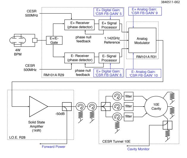
Figure 2.115: System overview of the longitudinal 14 ns feedback.
