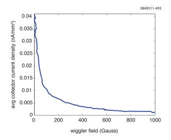
Figure 5.44: Wiggler ramp measurement in longitudinal field region: 1x45x.75 mA e+, 2.1 GeV, 14 ns
