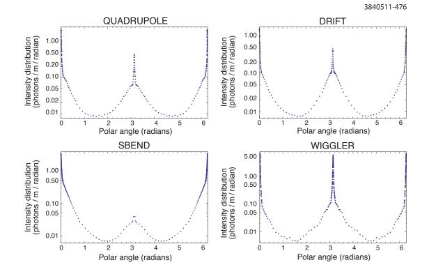
Figure 5.6: Photon intensity distribution (in photons/meter/radian) vs. polar angle (measured around the vacuum chamber, with zero angle corresponding to the radial outside direction), averaged over each type of magnetic environment. A 9 cm (horizontal) by 5 cm (vertical) elliptical vacuum chamber profile is assumed throughout the ring, and all scattering is specular. Top-bottom symmetry is assumed.
