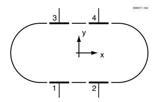
Figure 3.6: Button layout at a beam position detector
