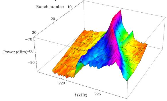
Figure 6.56: Data set 265: Bunch-by-bunch power spectrum: detail at horizontal betatron line, 4 GeV. Chromaticity: (H,V) = (1.3, 1.4). Bunch current = 1.1 mA.
