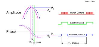
Figure 5.57: Steady state amplitude and phase response as the cavity resonant frequency changes from  $\omega_0$  to  $\omega_1$ .
