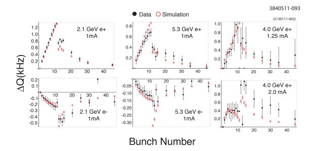
Figure 6.22: Vertical coherent tune shifts, 2010 data and POSINST simulations compared, using the parameters in Table 6.1.
