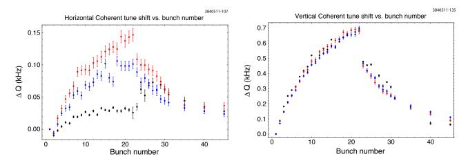
Figure 6.33: Tune shifts vs. bunch number, for 2.1 GeV data set corresponding to Fig. 6.19, left, computed (using POSINST) from Synrad (red points) and Synrad3D (blue) photon simulations, compared with data (black).
