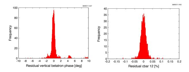
Figure 3.13: Reproducibility of vertical (left) betatron phase measurements, and transverse coupling (right).
