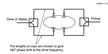
Figure 2.75: Signals from pairs of BPM electrodes are subtracted to improve coupling to the  $TE_{1,0}$  mode electric field and reject direct beam signal. At most locations, pairs are available for both excitation and/or detection of the waveguide modes.
