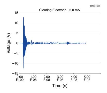
Figure 2.60: Clearing electrode HV port signal for a single 5 mA positron bunch
