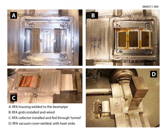
Figure 2.35: CESR dipole RFA assembly and welding photos.
