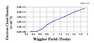
Figure 5.58: Estimate of EC density during a ramp of wigglers
