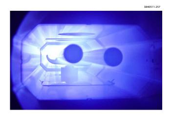
Figure 2.55: Glowing discharge during TiN coating of the grooved RFA beam pipe. The coating was performed in two stages, the first stage using two Ti rods (as shown) and the second stage with three rod (located in different transverse positions.) The two-stage coating is to minimize shadowing effects from the steeply grooved troughs.
