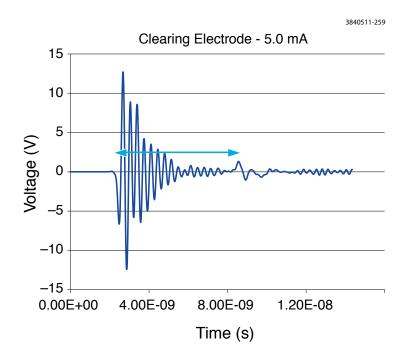
Figure 2.61: Clearing electrode HV port signal for a single 5 mA positron bunch on an expanded time scale. The time segment marked with the arrows represents the delay between signals induced at the HV coupling port end and the far end of the electrode.
