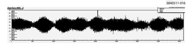
Figure 2.98: Beam position as a function of turn number for 4096 storage ring turns. Units are 50  $\mu$ m pixels measured at the image. The high frequency motion is due to betatron motion. In this example, with a maximum variation of ±4 pixels, and a magnification of 2.34, the beam motion at the source is ±85  $\mu$ m.
