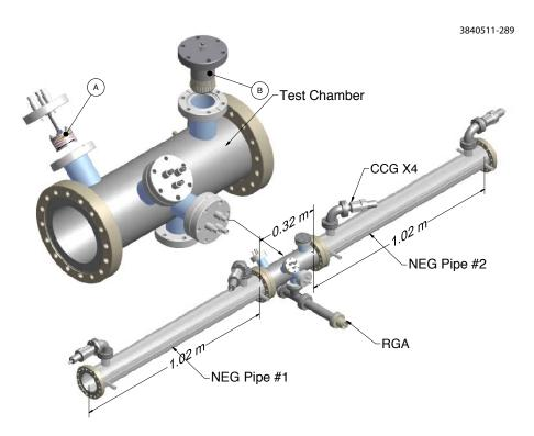
Figure 2.26: Vacuum chambers with NEG thin film coating in the drift section of the L3 experimental region. The test chamber included: (A) 3 units of APS-style RFAs; (B) RF-shielded pickup assembly supplied by LBNL.
