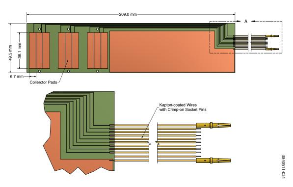
Figure 2.34: RFA flexible circuit collector for a CESR dipole chamber.
