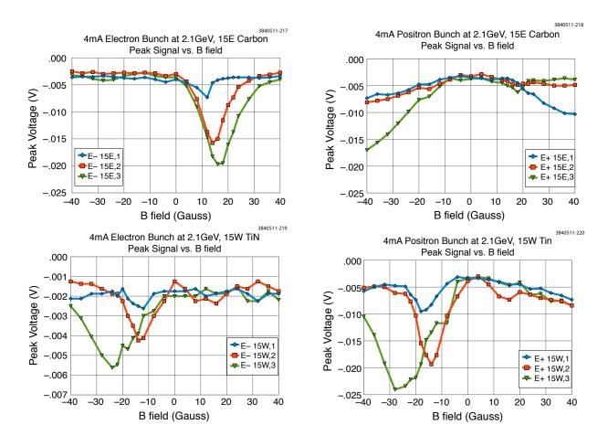
Figure 5.79: Pickup signal vs. solenoid field with a single bunch
