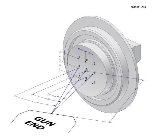
Figure 2.86: Isometric view of a sample showing the 9 grid points where the SEY is measured.
