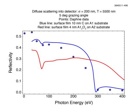
Figure 4.3: Diffuse scattering at 5 deg from a surface layer on an aluminum substrate: comparison of data and model
