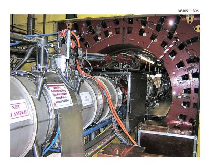
Figure 2.132: Wigglers in the wiggler straight section with their controls. The picture shows a view looking into the former CLEO detector with two of the three wigglers displayed to the left and the cabling of rightmost of these two in the center of the picture.
