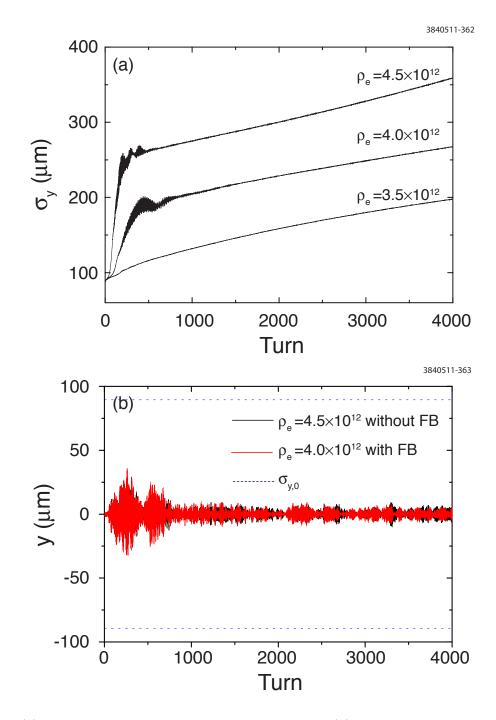
Figure 6.85: (a) Evolution of the beam size with feedback and (b) dipole moment with and without feedback at 5 GeV. The electron cloud density  $\rho_e$  is in units of m<sup>-3</sup>.
