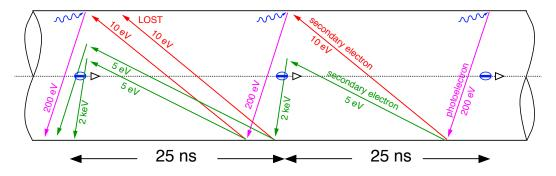
Figure 4.1: Cartoon illustrating the build-up of the electron cloud in the LHC for the case of 25-ns bunch spacing. The process starts with photoelectrons and is amplified by the secondary emission process. This cartoon was generated by F. Ruggiero.
