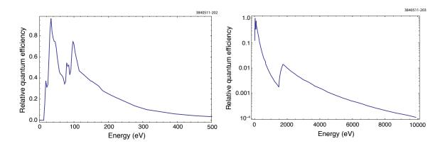
Figure 4.12: Relative quantum efficiency for an aluminum surface vs. photon energy. Left: energy range up to 0.5 keV. Right: energy range up to 10 keV. The L- and K-edges are evident at energies near 0.1 keV and 2 keV, respectively.
