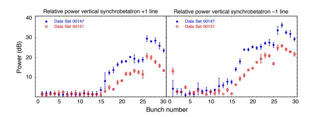
Figure 6.50: Data sets 147 and 151: vertical head-tail lines compared. Both sets have the same chromaticity [ (H,V) = (1.33, 1.16) ] and bunch current (0.74 mA), but different values of the bunch length and synchrotron frequency, as follows: 147,  $f_s = 25.4$  kHz and  $\sigma_z = 10.8$  mm; 151,  $f_s = 20.7$  kHz and  $\sigma_z = 12.8$  mm.
