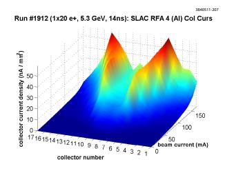
Figure 5.28: Bifurcation of peak cloud density in a Al dipole: 1x20 e+, 5.3 GeV, 14 ns
