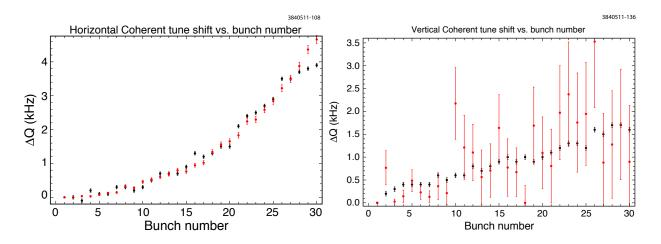
Figure 6.41: Data set 166 tune shifts: comparison between data (black) and simulation (red) from POSINST with parameters given in Table 6.1. Left: Horizontal tune shift vs. bunch number; right: Vertical tune shift vs. bunch number.
