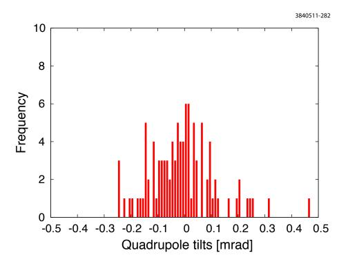
Figure 3.5: Distribution of measured tilt of ring quadrupoles with root mean square 133  $\mu$ rad.
