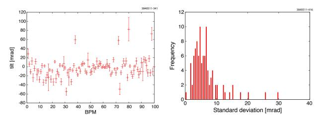
Figure 3.10: (Left) Measured BPM tilts. The error bars are  $\sigma = \frac{1}{N} \sqrt{\sum_{i=1}^{N} (\theta - \langle \theta \rangle)^2}$  of 58 data sets. (Right) The distribution of the rms residuals.
