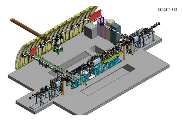
Figure 2.128: Final assembly drawing of the CESRTA beam line viewing L3 from above and the North and East. The pipes coming off of the CESR beam line to the south, transport the light from the vBSM's mounted just to the North (center of straight section) of the Q48W and Q48E quadrupoles (the outermost large blue magnets.)
