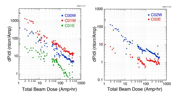
Figure 2.4: Beam induced pressure rise in the L0 EC experimental region during CHESS operations as a function beam dosage. The locations of the vacuum gauges are shown in Figure 2.3
