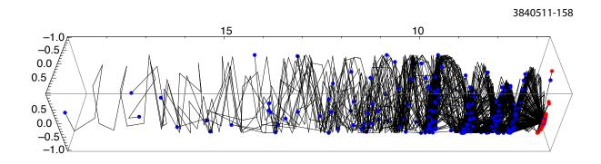
Figure 5.2: Photon trajectories from B12W in three dimensions. The photon source is on the right. Black lines are trajectories, and blue dots are photon absorption sites. The transverse geometry has been distorted from an ellipse to a circle, and the longitudinal dimension has been rectified and divided by 10, for purposes of illustration.
