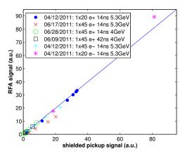
Figure 5.98: Comparison of RFA and SPU measurements, 15W TiN coated chamber. Each point represents a measurement with different beam current.
