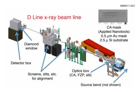
Figure 6.10: Layout of x-ray beam line for viewing positron beams at CESRTA.
