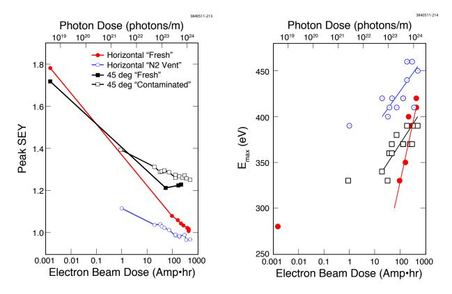
Figure 5.48: Dependence of SEY peak (left) and  $E_{\text{max}}$  (right) on dose for TiN-Al samples in the horizontal and  $45^{\circ}$  stations.
