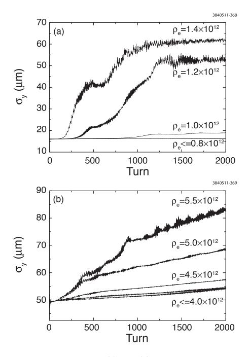
Figure 6.88: Evolution of the beam size in (a) 2 and (b) 5 GeV beam energies using the realistic lattices. The electron cloud density  $\rho_e$  is in units of m<sup>-3</sup>.
