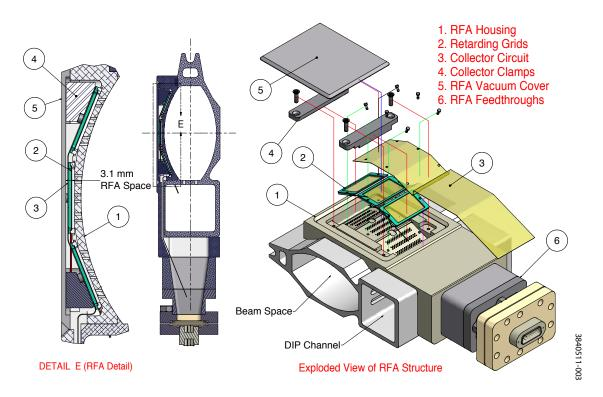
Figure 2.32: RFA design detail for a CESR dipole chamber.
