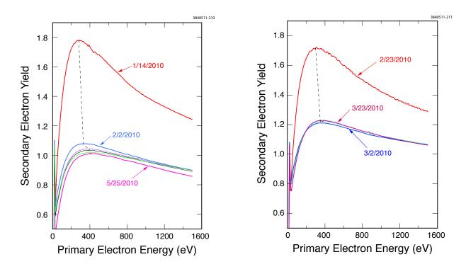
Figure 5.47: Repeated measurements of SEY as a function of energy for TiN-Al samples in the horizontal station (left) and the  $45^{\circ}$  station (right).
