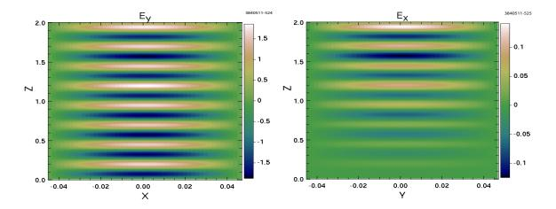
Figure 5.74: Transmission of a vertically-polarized TE wave in a square waveguide with a strong axial magnetic field and electron density of  $10^{15}$  m<sup>-3</sup>.
