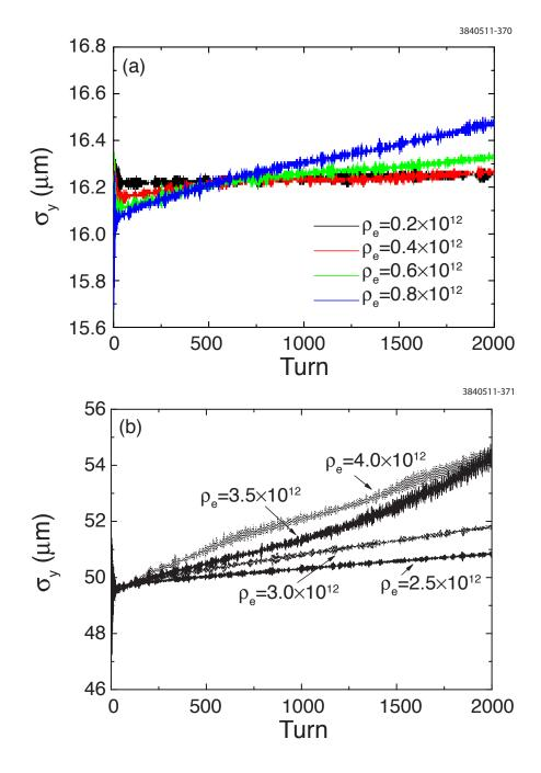
Figure 6.89: Evolution of the beam size below the threshold in (a) 2 and (b) 5 GeV beam energies. The electron cloud density  $\rho_e$  is in units of m<sup>-3</sup>.
