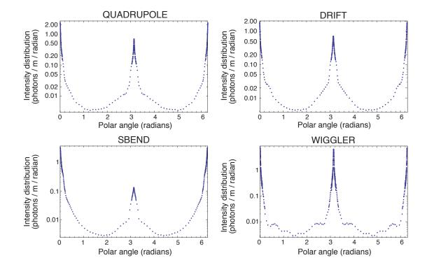
Figure 5.7: Photon intensity distribution (in photons/meter/radian) vs. polar angle (measured around the vacuum chamber, with zero angle corresponding to the radial outside direction), averaged over each type of magnetic environment. A realistic model for the CESRTA vacuum chamber throughout the ring is used. All scattering is specular. Top-bottom symmetry is assumed.
