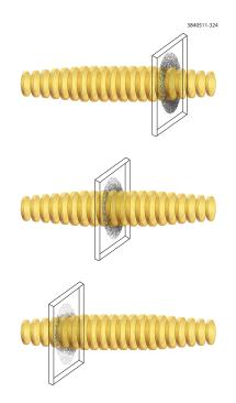
Figure 6.14: Figure describing the pinching of the cloud as the slices of the beam pass through the two dimensional cloud
