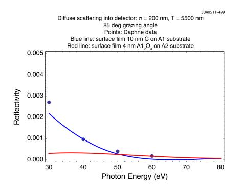
Figure 4.5: Diffuse scattering at 85 deg from a surface layer on an aluminum substrate: comparison of data and model
