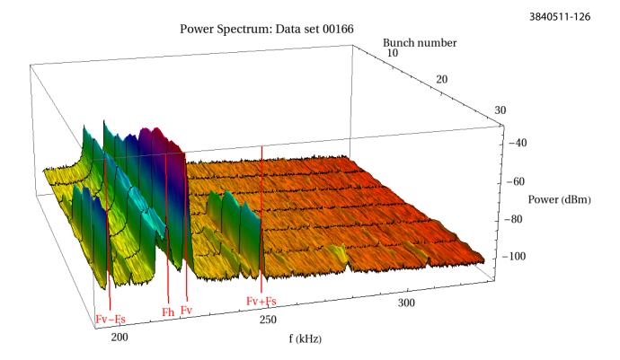
Figure 6.36: Data set 166: Bunch-by-bunch power spectrum
