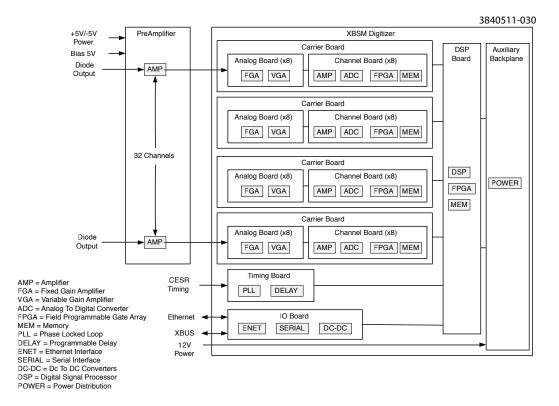
Figure 2.94: xBSM data acquisition system
