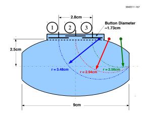
Figure 5.96: Vacuum chamber wall cross section with circular trajectories of photoelectrons contributing to the pickup signals.
