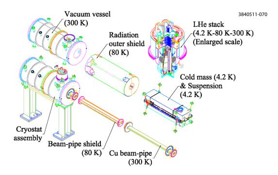
Figure 2.38: Exploded view of the structure of a CESR-c superconducting wiggler assembly.
