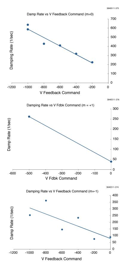
Figure 6.67: Single bunch damping rate vs. vertical dipole feedback. Top: vertical m = 0 mode. Center: vertical m = +1 head-tail mode. Bottom: vertical m = -1 head-tail mode.
