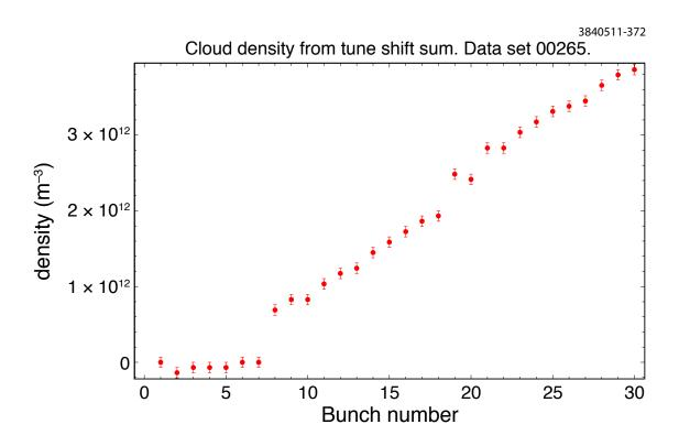
Figure 6.59: Data set 265: Average initial electron cloud density vs. bunch number, estimate from measured tune shifts. 4 GeV beam energy.
