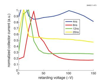
Figure 5.17: Resonant spike location at different bunch spacings, 45 bunches, 1.25 mA/bunch, e+, 5 GeV. Only the signal in the central collector is plotted
