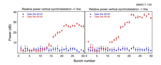
Figure 6.46: Data sets 142 and 150: vertical head-tail lines compared. Both sets have the same chromaticity [ (H,V) = (1.34, 1.99) ] but different bunch currents as follows: 142: 0.74 mA; 150: 0.95 mA
