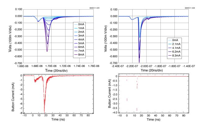
Figure 5.80: Upper row: shielded pickup signals produced by two 5.3 GeV positron (left) and electron (right) bunches separated by 14 ns. The leading bunch population is  $1.3 \times 10^{11}$ , or 8.2 mA. The population of the second bunch varies up to a similar value. Lower row: initial ECLOUD model results exhibiting discrepancies with the measured signals which are quite dramatic in the case of the electron beam.
