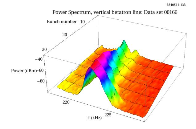
Figure 6.39: Data set 166: Bunch-by-bunch power spectrum: detail at vertical betatron line. Chromaticity: (H,V) = (1.33, 1.16). Bunch current = 0.74 mA.
