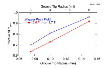
Figure 2.52: Simulated effective peak SEY on triangular grooves on copper as a function of groove tip/valley radius (sharpness) for two typical wiggler peak fields. (The simulation assumed the tips and valleys to have the same radius.) The two peak wiggler fields correspond to CESR beam energies of 1.8 GeV and 5.2 GeV.
