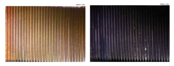
Figure 2.56: The grooves of the SCW RFA beam pipe were inspected optically. LEFT: Before TiN coating; RIGHT: After TiN coating.
