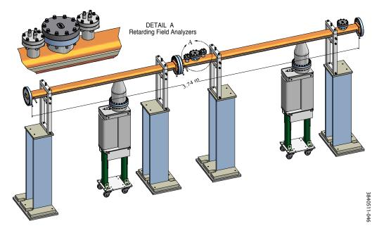
Figure 2.8: EC experiment section created by the removal of SCW-doublets in CESR.
