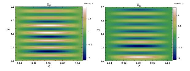
Figure 5.75: Transmission of a vertically-polarized TE wave in a square waveguide with vertical polarization and an axial magnetic field near resonance. The electron density is  $10^{15}$  m<sup>-3</sup>. A left-hand circularly polarized wave is transmitted at roughly half the original power.
