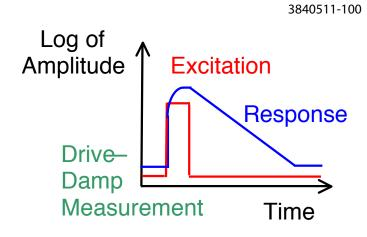
Figure 6.11: Illustration of the drive-damp measurement: The red trace is the amplitude of the excitation driving the bunch. The blue trace is the bunch response.
