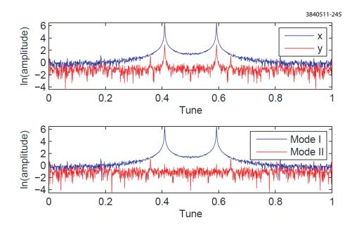
Figure 3.16: Fourier spectra of turn-by-turn signals recorded on BPM 7W. Top: "nominal" (x-y) calibration, showing peaks corresponding to the mode I frequency in both x and y coordinates. Bottom: "normal mode" calibration, showing the normal mode frequencies appearing in only the corresponding normal mode coordinate.
