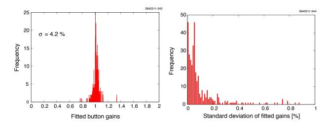
Figure 3.9: (Left) Distribution of measured button gains, with standard deviation 4.2%. (Right) Distribution of the variation in fitted button gains for seven sets of turn by turn data.
