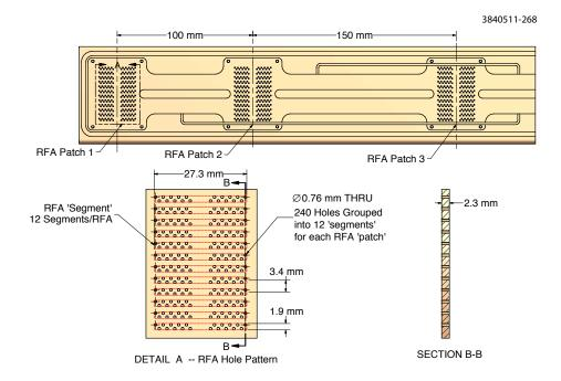
Figure 2.42: Small holes are drilled through top beam pipe to allow electrons in the beam pipe drift into RFAs. There are 240 holes for each RFA, and they are grouped into 12 segments to sample transverse EC density distribution.
