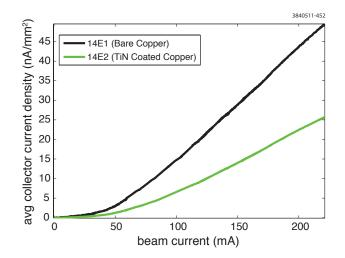
Figure 5.20: Comparison of insertable drift RFAs, 1x20 e+, 5.3 GeV, 14 ns
