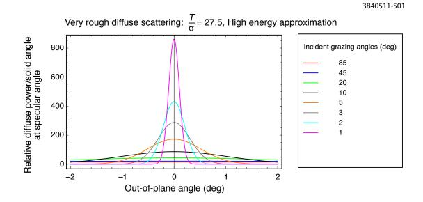
Figure 4.10: Diffuse scattering out-of-plane angular distributions for high energy photons
