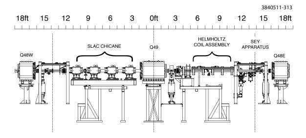
Figure 2.125: Schematic layout of the L3 experimental region. The experimental area includes the following vacuum chamber test regions: a chicane section, a region that has Helmholtz coils around the beam pipe to allow for chamber processing via bakeout etc., and an SEY apparatus with a lock-load mechanism to permit easy access for changing vacuum chamber wall surfaces.
