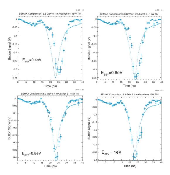
Figure 5.87: Modeled and measured two-bunch signals with values for the parameter  $E_{\text{SEY}}$  ranging from 0.4 to 1.0. For values of  $E_{\text{SEY}}$  less than 0.8, the model is inconsistent with the measured witness-bunch signal.
