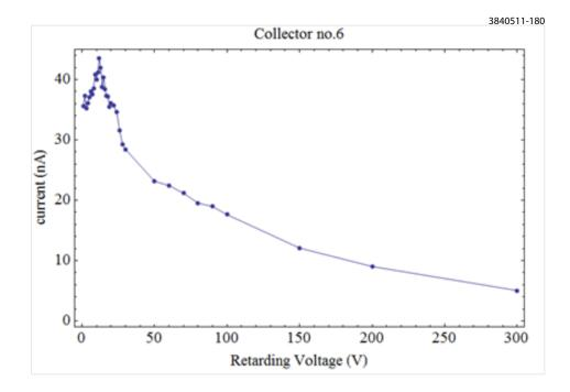
Figure 5.18: POSINST simulation showing resonant enhancement, 45 bunches, 1.2 mA/bunch, e+, 2.1 GeV, 14 ns, central collector
