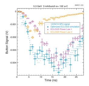
Figure 5.84: Two power-law contributions to the modeled photoelectron energy distribution. The yellow circles show the contribution to the signal from the high-energy photoelectron component, and the magenta triangles the low-energy contribution. The combined result is shown in blue.
