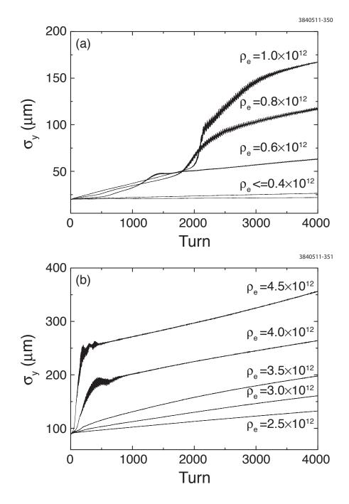
Figure 6.80: Evolution of vertical beam size growth for various cloud densities in CESRTA (a) 2 and (b) 5 GeV beam energies. The electron cloud density  $\rho_e$  is in units of m<sup>-3</sup>.
