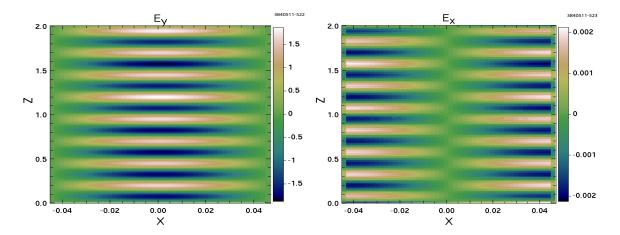
Figure 5.73: Transmission of a vertically-polarized TE wave in a square waveguide with a strong horizontal magnetic field and electron density of  $10^{15}$  m<sup>-3</sup>.
