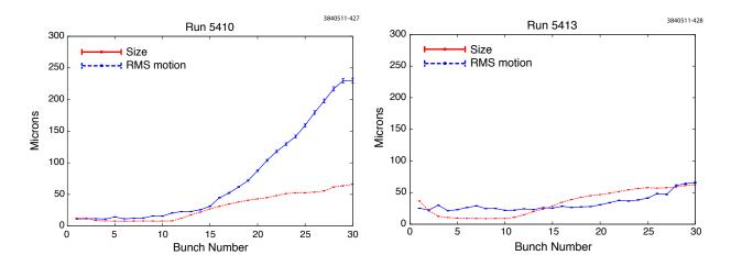
Figure 6.74: Bunch-by-bunch beam size and rms motion at 14 ns spacing, 0.75 mA/bunch. Left: vertical chromaticity  $\sim 1.2$ . Right: vertical chromaticity  $\sim 2.2$ .
