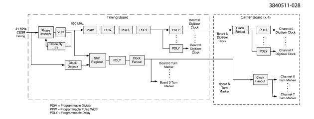
Figure 2.96: xBSM internal timing
