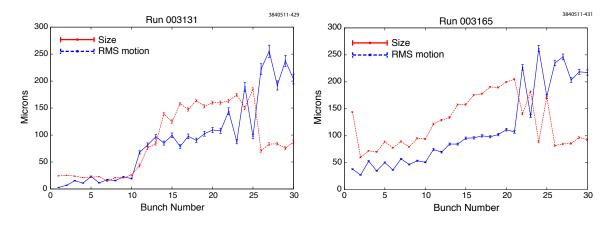
Figure 6.76: Bunch-by-bunch beam size and rms motion at 4 ns spacing with 0.75 mA/bunch. Left: nominal emittance. Right: increased initial emittance.
