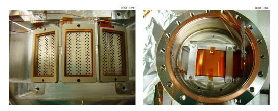
Figure 2.17: Photos of the Cornell Dipole thin-style RFA taken while it was being installed into the Q15 experimental chamber. Left: the three high-transparency retarding grids after installation onto the beam pipe. The beam pipe holes are clearly visible through the fine meshes of the grids. Right: installation of the collector circuit, which is clamped down with aluminum bars.
