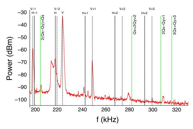
Figure 6.37: Data set 166: Power spectrum for bunch 30. The lines labelled, for example, "V+1" and "V-1" are shown at frequencies of  $\pm f_s$  from the vertical betatron line ("V"), in which  $f_s$  is the synchrotron frequency. The locations of several machine resonances are also indicated.
