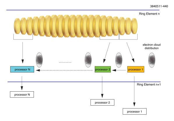
Figure 6.17: Figure illustrating the flow of information for parallel computation implemented in CMAD
