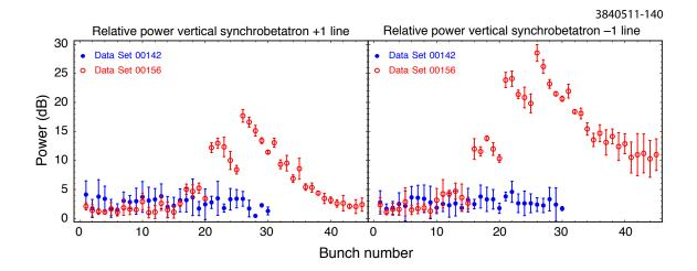
Figure 6.48: Data sets 142 and 156: vertical head-tail lines compared. Both sets have the same chromaticity [ (H,V) = (1.34, 1.99) ] and bunch current (0.74 mA), but different numbers of bunches, as shown in the figure. The increased amplitude in data set 156 at bunches 21 and 26 is an artifact due to refilling of the train at these bunch numbers.
