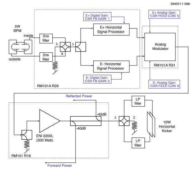
Figure 2.114: System overview of the horizontal 14 ns feedback.
