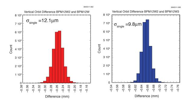
Figure 2.91: Vertical orbit differences between closely located detectors
