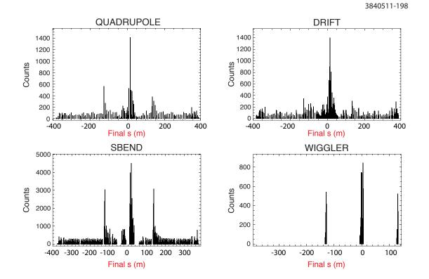
Figure 5.5: Distribution of photon absorption sites vs. longitudinal position, for different magnetic environments. The origin for the longitudinal coordinate is the center of the L0 straight section. The ring circumference is about 760 m.
