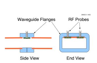
Figure 5.60: Sketch of straight drive flange
