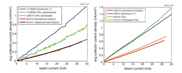
Figure 5.24: Comparison of different beam pipe coatings, 15E (left), and 15W (right) drift RFAs. Plots show average collector signal vs beam current for **9** equally spaced (**280** ns) bunches of **positrons**, at beam energy **5.3 GeV**. Note that the aluminum chamber signals are divided by 3.
