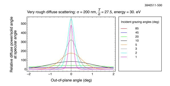
Figure 4.8: Diffuse scattering out-of-plane angular distributions for 30 eV photons
