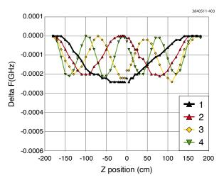
Figure 5.61: Multiple half-wavelength resonances are observed in a section of WR284 waveguide.
