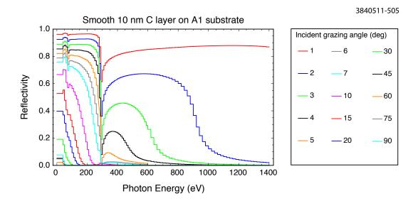
Figure 4.6: Smooth surface reflectivity for a 10 nm C film on Al substrate: from [95]
