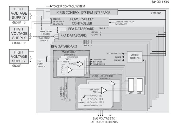
Figure 2.71: Schematic showing the high voltage power supply system and the RFA current monitor boards.
