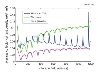
Figure 5.29: RFA signal as a function of chicane magnetic field: 1x45x1 mA e+, 5 GeV, 4 ns. Cyclotron resonances are observed every 89 G. Note that the Aluminum chamber signal is divided by 20.
