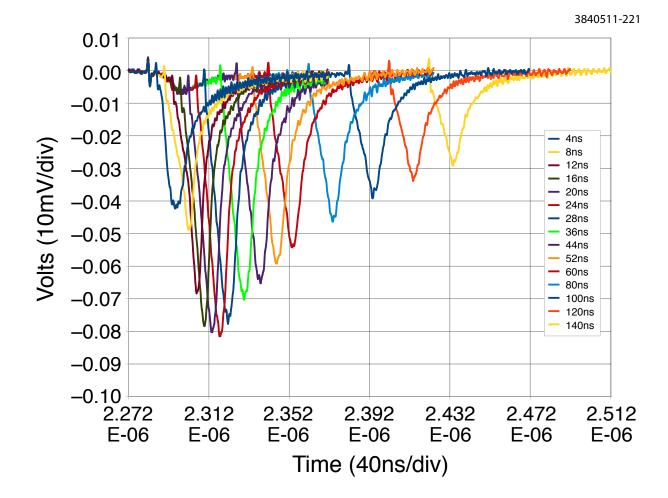
Figure 5.78: Overlay of two bunch data with spacings in multiples of 4 ns at 2.1 GeV with an aluminum chamber
