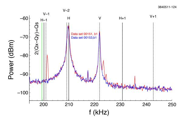
Figure 6.62: Data set 151 and 153 : Power spectrum, bunch 1, compared. Both sets have the same chromaticity and bunch current, but there is a precursor bunch present for data set 153, as described in the text. The lines labelled, for example, "V+1" and "V-1" are shown at frequencies of  $\pm f_s$  from the vertical betatron line ("V"), in which  $f_s$  is the synchrotron frequency. For these data sets,  $f_s = 20.7$  kHz. The location of a machine resonance is also indicated.
