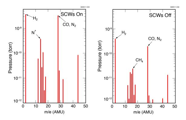
Figure 2.5: RGA spectra at L0 Center, with 120 mA positron at 4-GeV, with SCWs ON (left) and OFF (right). The relative peak heights of signals at  $\frac{m}{e} = 28$  and 14 clearly indicated desorption of N<sub>2</sub> with SCWs on, due to higher energy SR photons.
