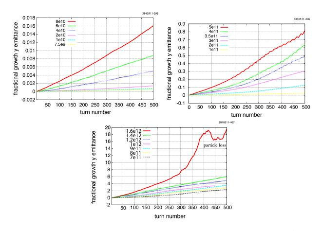
Figure 6.92: Vertical emittance growth rate for varying cloud densities, in units of  $m^{-3}$ .
