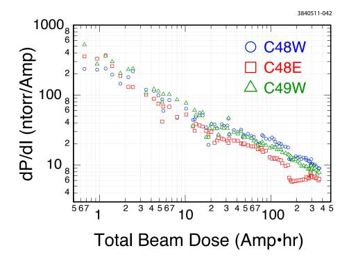
Figure 2.11: Typical vacuum beam conditioning performance for the L3 experimental region
