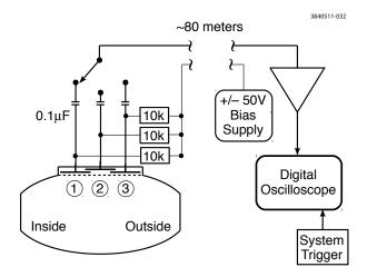
Figure 2.83: The shielded pickup signal is selected with a relay and routed to amplifiers and oscilloscope.
