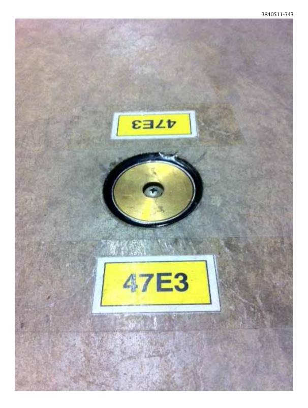
Figure 2.119: Floor target.
