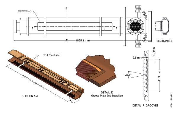
Figure 2.50: SCW RFA beam pipe with a groove plate EB welded to the bottom beam pipe.
