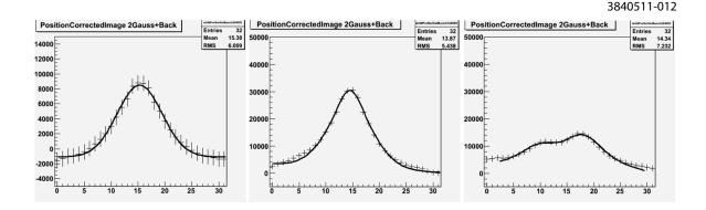
Figure 2.103: Typical image for pinhole, Fresnel Zone Plate and coded aperture, with beam sizes  $80 \ \mu m$ ,  $40 \ \mu m$  and  $60 \ \mu m$  respectively.
