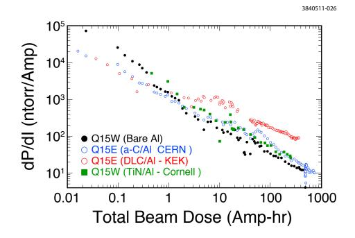
Figure 2.15: History of beam-induced vacuum conditioning of four Q15 EC test chambers with different surfaces.
