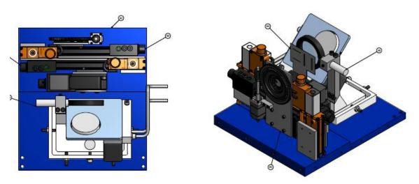
Figure 2.105: Visible synchrotron light monitor optics box. The optics box contains an aris with adjustable aperture, a double slit, a lens, and a mirror.
