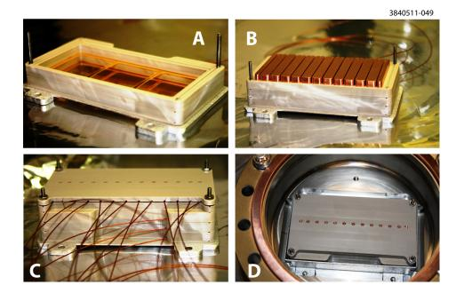
Figure 2.18: Photographs of insertable RFA used in Q15 experimental chambers. (A) Hightransparency gold-coated copper meshes after mounting in PEEK frames. (B) Copper bar collectors mounted above the meshes. (C) RFA assembly with PEEK top cap, after soldering all connections (including 2 grids and 13 collectors). (D) Insertable RFA in the vacuum port of a test chamber (for clarity, wires are not shown).
