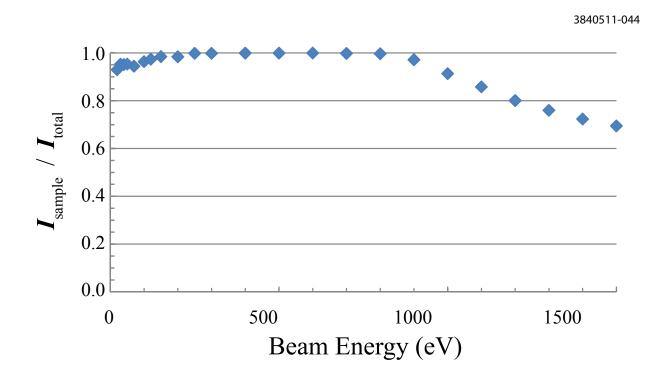
Figure 2.88: Slit collimation measurements for the SEY system. For the vertical axis,  $I_{sample}$  is the current reaching the sample and  $I_{total}$  is the current reaching the sample plus the current reaching the collimation electrode.
