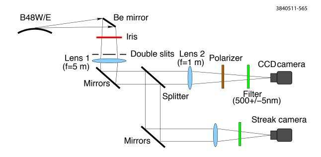
Figure 2.104: Visible synchrotron light monitor optics.
