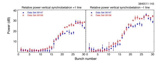
Figure 6.51: Data sets 147 and 158: vertical head-tail lines compared. Both sets have the same chromaticity [ (H,V) = (1.33, 1.16) ] and bunch current (0.74AmA), but different values of the single-bunch vertical emittance, as follows: 147, Vertical emittance  $\sim 20$  pm; 158, Vertical emittance  $\sim 300$  pm
