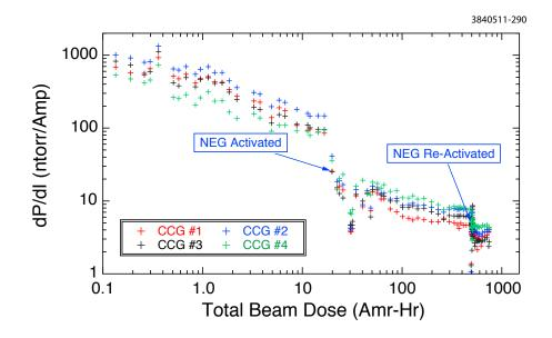
Figure 2.29: Beam conditioning of the NEG coated beam pipes in L3.
