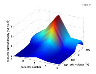
Figure 5.19: RFA voltage scan with an insertable segmented drift RFA in a Cu chamber, 1x45x1.25 mA e+, 14 ns, 5.3 GeV
