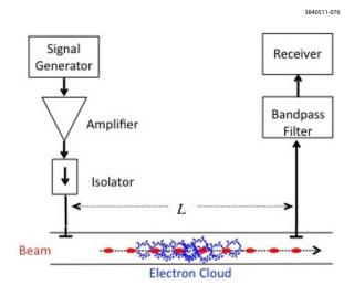
Figure 2.74: Schematic view of the TE-wave transmission technique for measuring the electron cloud density.
