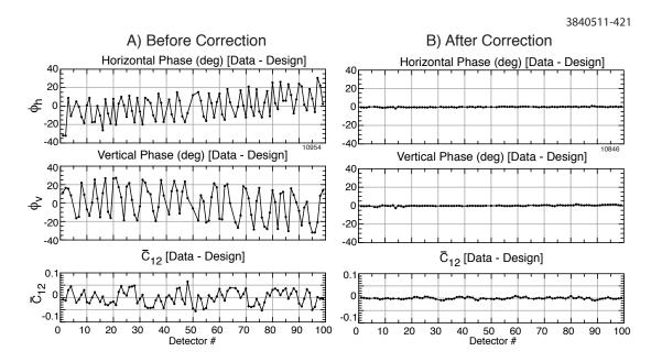
Figure 3.7: Example betatron phase and coupling correction. A) Measured betatron phase and  $\overline{C}_{12}$  coupling matrix element before a correction. Plotted are the difference between the measured values and the design values as computed from the theoretical design lattice. B) Measured values after correction. A perfect correction would result in the measured values being equal to the design ones.
