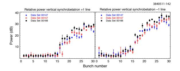
Figure 6.44: Data sets 147, 157 and 166: vertical head-tail lines compared. All sets have the same nominal bunch current and chromaticity.
