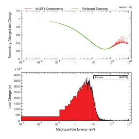
Figure 5.34: Population of the modeled secondary yield curve for the case of a TiNcoated aluminum chamber and a chicane magnetic field value of 129 G, halfway between the first and second cyclotron resonances for the 4-ns bunch spacing.
