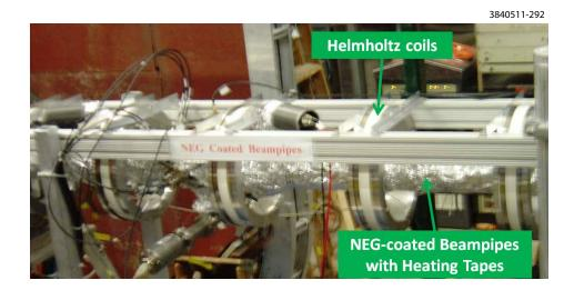
Figure 2.28: NEG-coated beam pipes in L3 after installation of Helmholtz Coils.
