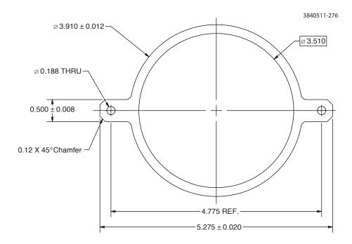
Figure 2.19: Cross section of PEP-II aluminum beam pipe with a smooth interior wall. The beam pipe was extruded with type 6063-T6 aluminum alloy.
