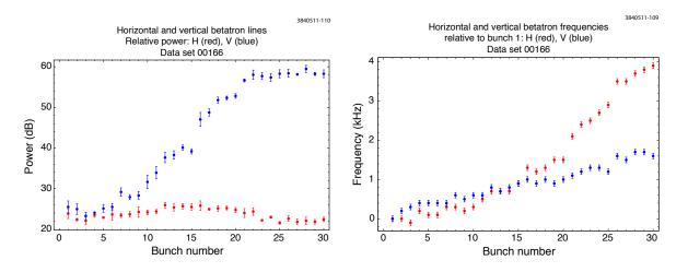
Figure 6.40: Data set 166: Left, Horizontal and vertical peak power vs. bunch number; right, Horizontal and vertical tune shifts vs. bunch number. Chromaticity: (H,V) = (1.33, 1.16). Bunch current = 0.74 mA.
