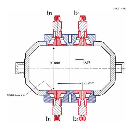
Figure 2.89: BPM module functional diagram
