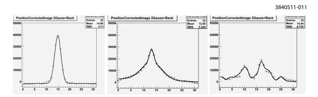
Figure 2.97: Typical images for pinhole, Fresnel zone plate and coded aperture, each with 16  $\mu m$  beam size.
