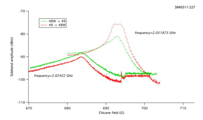
Figure 5.64: Modulation sideband amplitude near the upper hybrid resonance at two different frequencies. Red and green traces correspond to opposite direction of propagation of the TE wave.
