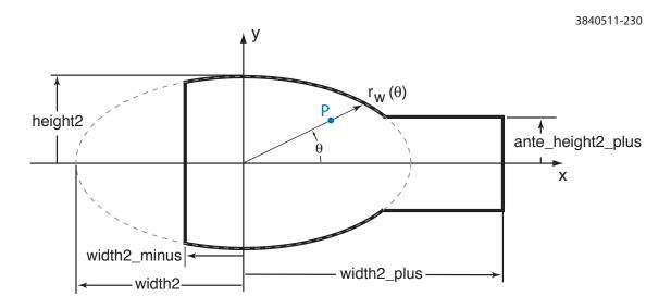
Figure 4.11: Vacuum chamber model
