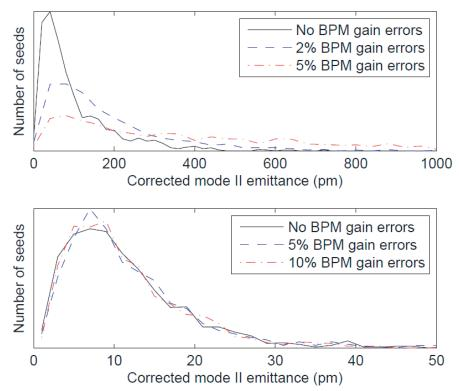
Figure 3.17: Results of simulation of low-emittance tuning in CESRTA using: (top) correction of vertical orbit and vertical dispersion; (bottom) correction of mode II dispersion, using BPMs calibrated to measure beam motion in the normal modes. The lines show the distribution of final mode II emittance over 1000 seeds of random machine errors, for different cases of BPM gain errors.
