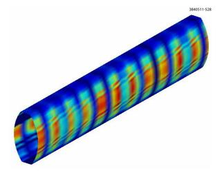
Figure 5.65: Snapshot of a vorpal simulation showing propagation of a TE wave through the CESRTA beam pipe
