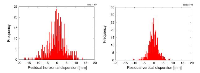
Figure 3.12: Reproducibility of horizontal (left) and vertical (right) dispersion measurements. The standard deviation of the measurements is 4.6 mm and 2.3 mm respectively.
