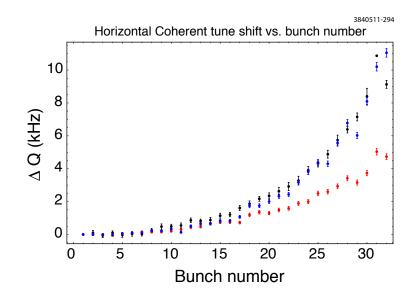
Figure 6.24: Horizontal coherent tune shifts, Dimel data (black) and POSINST simulations (red, blue) ("Modified static cloud model") compared. 32 bunch train, 0.8 mA bunch current, 2.1 GeV beam energy, 4 ns bunch spacing. Red: POSINST simulation using parameters given in Table 6.1. Blue: same simulation parameters except total peak secondary yield = 2.3
