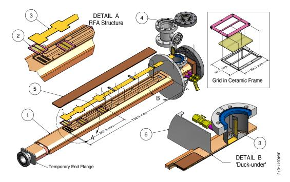
Figure 2.40: Exploded View of a SCW RFA beam pipe Assembly. The key components are: (1) beam pipe top half, housing the RFAs; (2) RFA grids (see upper right inset); (3) RFA collector on a flexible printed circuit board; (4) RFA connection port; (5) RFA vacuum cover. The 'duck-under' channel, through which the kapton flexible circuit is fed after all heavy welding is complete, is shown in detail B.
