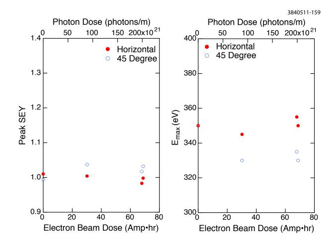
Figure 5.50: Dependence of SEY peak (left) and  $E_{\text{max}}$  (right) on dose for amorphous carbon-coated samples in the horizontal and  $45^{\circ}$  stations.
