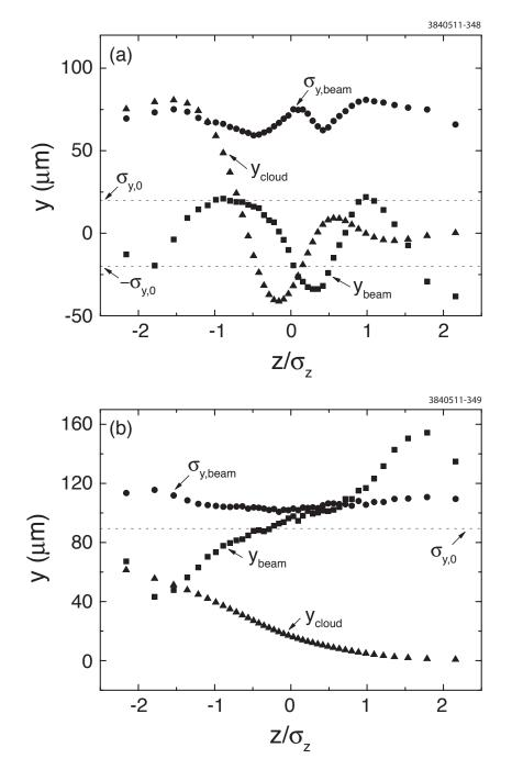
Figure 6.79: The vertical position and size of the bunch slices and the vertical position of the electron cloud interacting with the slices above the threshold are depicted for (a) 2 and (b) 5 GeV beam energies. The dotted lines indicate the initial vertical beam sizes. The head of the bunch is at z > 0.
