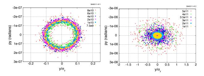
Figure 6.93: Vertical phase space for varying cloud densities, in units of  $m^{-3}$ .
