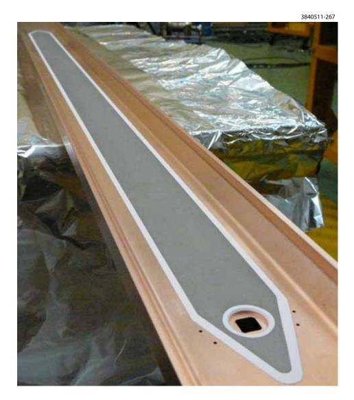
Figure 2.58: Photo of deposited electrode on the bottom of the SCW beam pipe.
