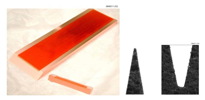
Figure 2.53: LEFT: A prototype groove plate was fabricated with full-hard OFC copper. A precision wire-cut across the grooves was performed for groove sharpness inspection. RIGHT: Images of prototype groove tip and valley, taken with a high-resolution camera on the CMM at LBNL with back-lighting. The tip radius is estimated to be approximately 0.001" (25  $\mu$ m) and the valley approximately 0.0025" (63  $\mu$ m). (Photo courtesy of Dawn Munson of LBNL)
