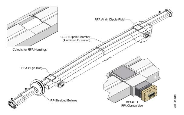
Figure 2.31: A CESR dipole chamber with 2 RFAs.
