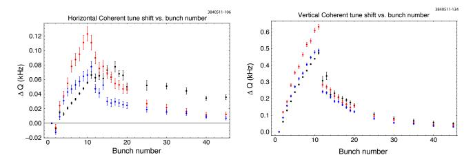
Figure 6.34: Tune shifts vs. bunch number, for 5.3 GeV data set corresponding to Fig. 6.20, left, computed (using POSINST) from Synrad (red points) and Synrad3D (blue) photon simulations, compared with data (black).
