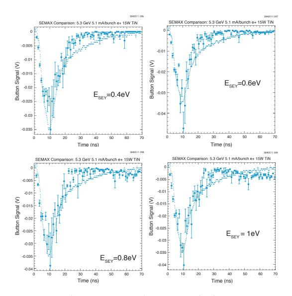
Figure 5.86: Modeled (points with error bars) and measured (dots) leading SPU signals with differing distributions for the parameter  $E_{\text{SEY}}$  ranging from 0.4 to 1.0. For values of  $E_{\text{SEY}}$  greater than 0.8, the modeled signal exhibits a tail at later times inconsistent with the measured signal.
