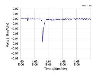
Figure 5.77: The signal from two bunches of electrons spaced at 20 ns
