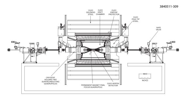
Figure 2.121: An elevation view of the CESR-c/CLEO-c interaction region before reconfiguration as the wiggler straight section for CESRTA. The central section of the CLEO-c detector, the final focusing superconducting quadrupoles and the connecting vacuum chambers were removed during the CESRTA installation.
