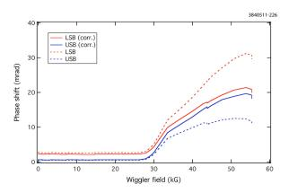
Figure 5.55: Sideband levels relative to the carrier during wiggler ramp in the L0 straight with (solid lines) and without (dashed) correction applied.
