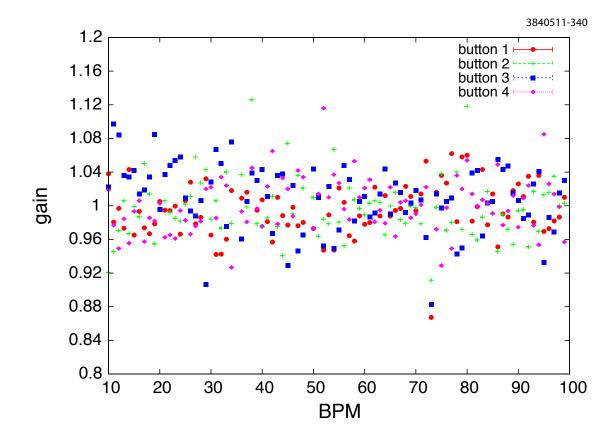
Figure 3.8: Measured BPM button gains. Note that there are four data points for each BPM.
