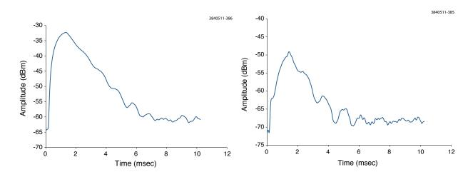
Figure 6.65: Plot of the amplitude vs. time for a drive-damp measurements. Left: m = 0 mode. Right: m = -1 mode.
