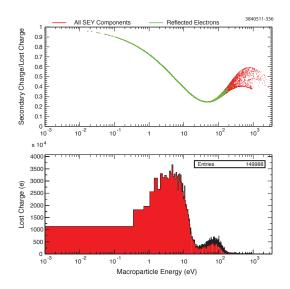
Figure 5.35: Population of the modeled secondary yield curve for the case of an TiNcoated aluminum chamber and a chicane magnetic field value of 89 G, which corresponds to the first cyclotron resonance for the 4 ns bunch spacing.
