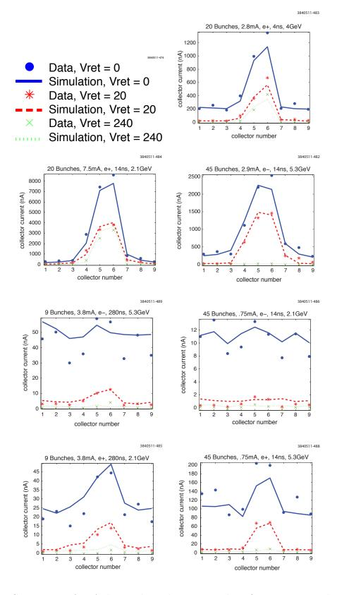
Figure 5.45: Comparison of RFA data and simulation, using best fit parameters. The plots show the signal across the 9 RFA collectors at three different retarding voltages.
