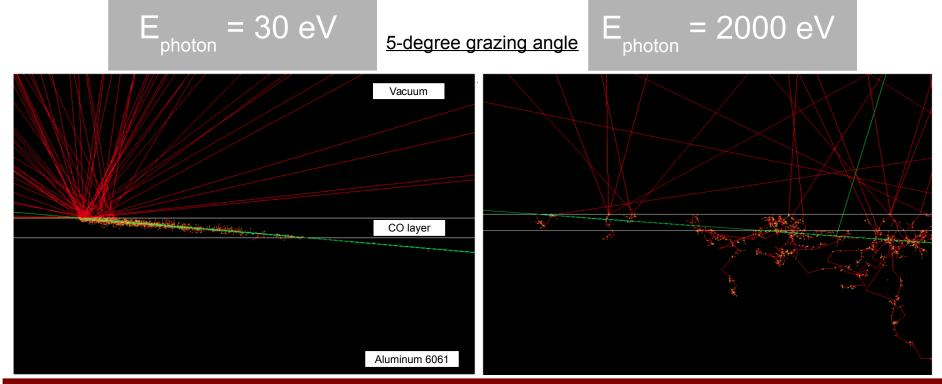
Zoom in on the 5-nm CO layer. Low-energy photons interact predominantly in the CO layer. High energy photons are absorbed most frequently in the aluminum
