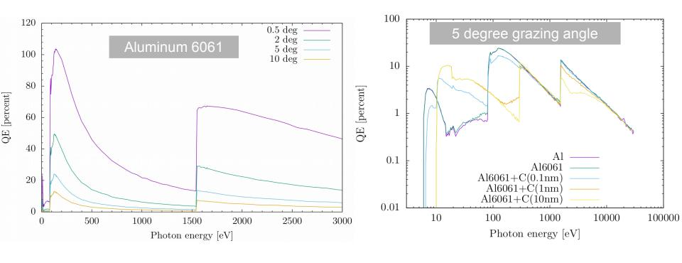
Geant4 photoabsorption cross sections show important dependence on absorbed photon energy and angle of incidence on the wall.
