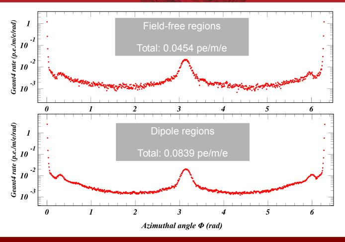
Number of electrons per beam particle per meter provided to electron cloud buildup modeling in 720 azimuthal location bins averaged over dipole and field-free regions separately.
