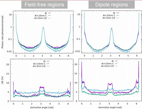
Product of quantum efficiency and photon rate used as input to electron cloud buildup model (e-/m/e+ vs azimuthal angle)
