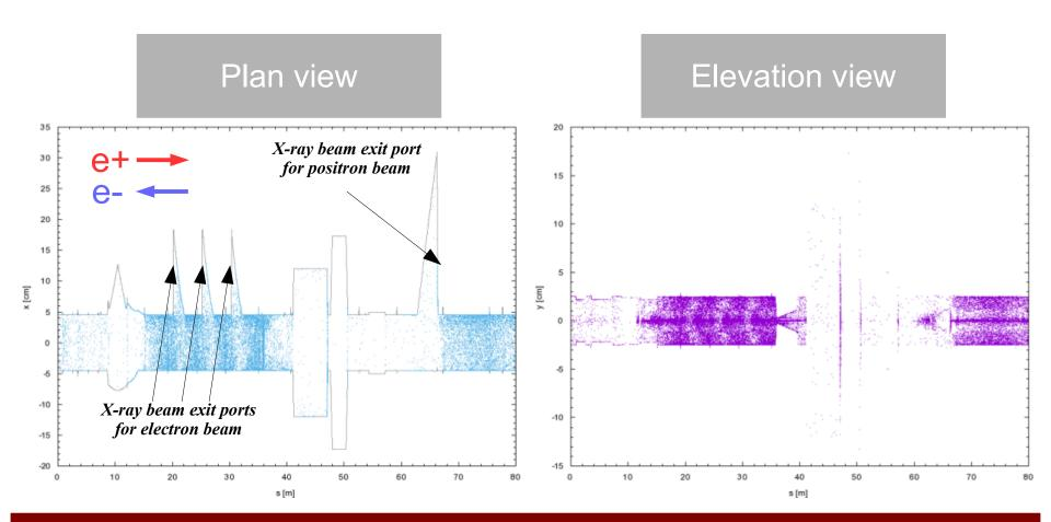
10<sup>6</sup> photons tracked around the 768-m CESR ring Vacuum chamber model includes gate valves, bellows, etc
