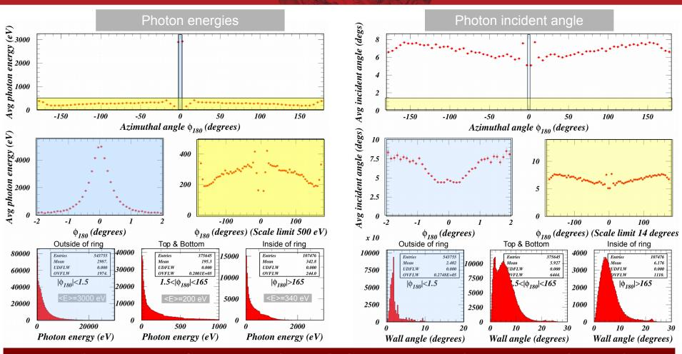
Dramatic dependence of photon energies and incident angles on azimuthal absorption location.
