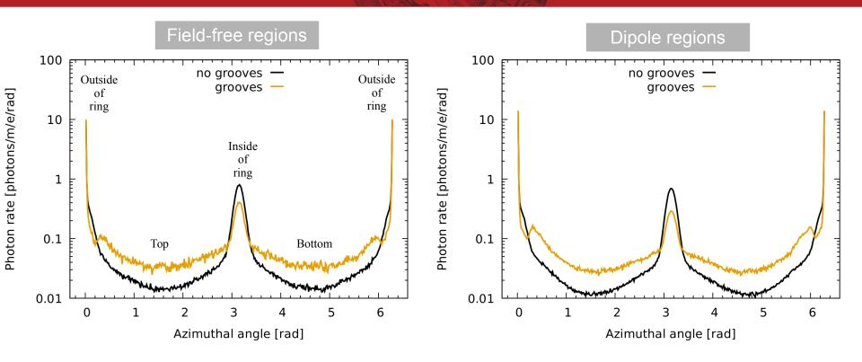
The effect of grooves is to enhance photoelectron production on the top and bottom of the beam-pipe, increasing the contribution of dipole regions to the tune shift and emittance growth calculations due to the tight spiraling of cloud electrons around the vertical magnetic field lines guiding them into the beam.
