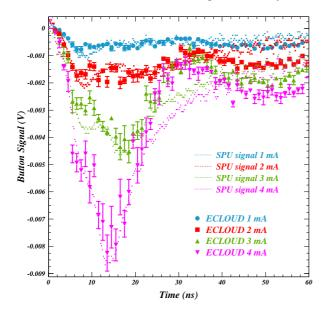
Figure 5: Single bunch signal dependence on positron bunch population. The small symbols show the digitized SPU signal. The larger symbols with error bars show the ECLOUD-modeled signal and its associated statistical uncertainty arising from counting signal macroparticles in each time bin. As the bunch population increases, the beam kick increases the contribution to the SPU signal from photoelectrons produced with lower kinetic energy.
