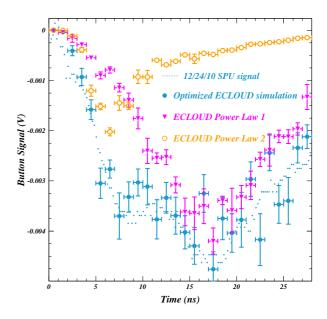
Figure 6: Contributions to the modeled signal from simulations including a single power law contribution (orange circles show the higher energy contribution, pink triangles show the lower energy contribution) as well as the simulation including the weighted sum of the two distributions which provides the observed degree of consistency with the measured signal shape.
