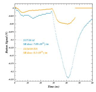
Figure 4: Comparison of signals recorded in May and December 2010 in an uncoated aluminum chamber and in a TiN-coated chamber, whereby the populations of the two positron bunches are  $4.8 \times 10^{10}$ .
