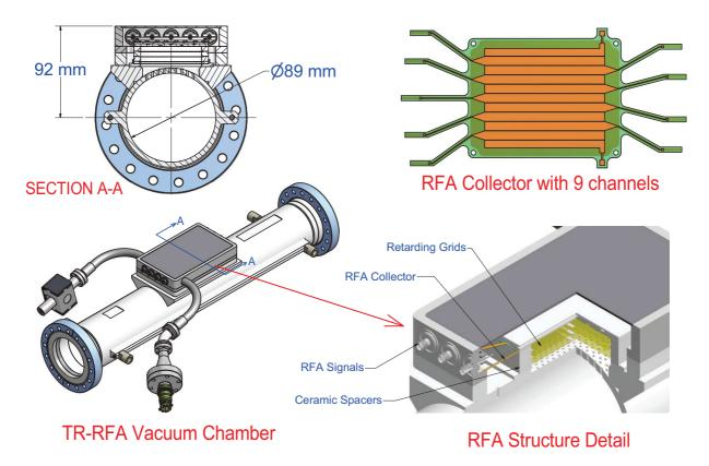
Figure 14: Engineering drawings of a CESRTA time-resolved retarding field analyzer. The two drawings in the left column show the 8.9-cm-diameter custom vacuum chamber on which the TR-RFAs are installed. The nine collectors are arranged as shown on the upper right. The interior grid structure is shown on the lower right.
