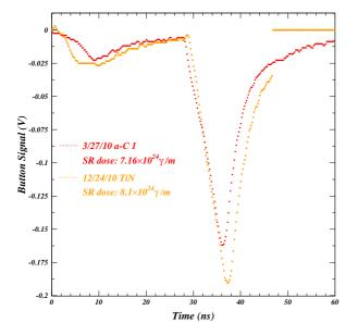
Figure 3: Examples of SPU signals produced by two bunches of  $8\times 10^{10}$  5.3 GeV positrons spaced 28 ns apart. The top figure compares signals recorded in March and December of 2010 for two vacuum chambers in the same position in CESR ring. The amorphous-carbon-coated and TiN-coated aluminum chambers have each been well-conditioned by a synchrotron radiation dose of about  $8\times 10^{24}\gamma/m$ .
