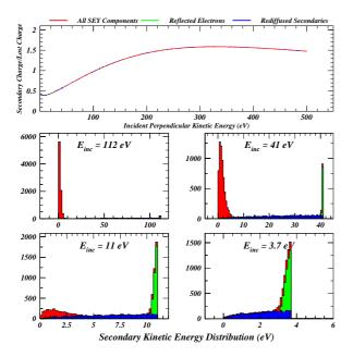
Figure 8: Example of the secondary emission model implemented in the ECLOUD code. The top plot shows the total yield curve including the contributions from the true secondary, re-diffused and elastic processes. The lower four plots show the energy distributions of the secondaries in the case of perpendicular incidence for electrons of energy 112, 41, 11 and 3.7 eV.
