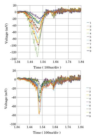
Figure 15: Signals from the nine TR-RFA collectors in the aluminum vacuum chamber without grooves. A train of ten bunches of 5.3 GeV positrons of population  $1.3\times10^{11}$  is followed by one witness bunch 112 ns after the train. The upper plot shows the case for no dipole field. The lower plot shows the effect of a 45 G field, which results in a central depletion zone in the cloud.
