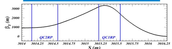
The cloud causes vertical focusing via the space charge field gradient. Owing to the very high beta function, the fractional tune shift value of 0.16 is about a factor of 15 higher than caused by the cloud in the entire rest of the ring.
