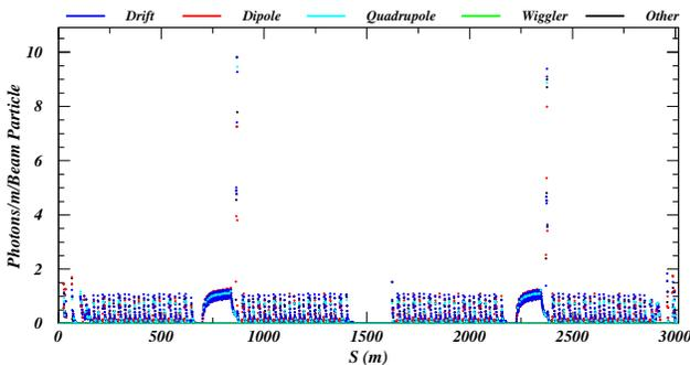
Figure 4: Analytic calculation of the synchrotron radiation pattern directly incident on the outside wall of the 4-GeV positron ring. The lattice element type in which the photons strike the wall is color-coded as shown.
