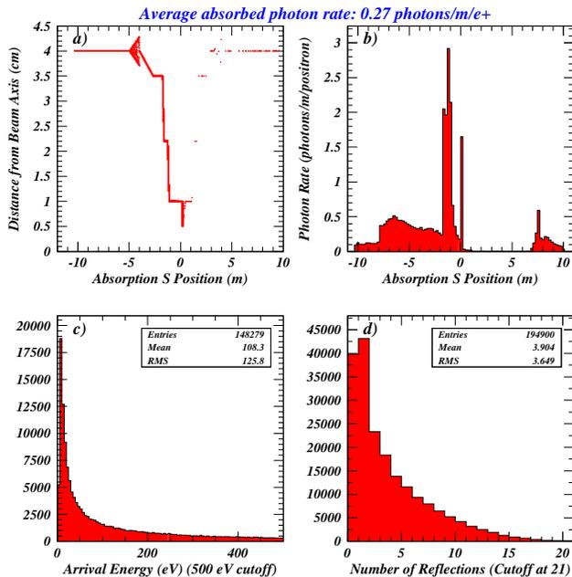
Figure 6: Distributions of photons absorbed within 10 m of the IP. a) Scatter plot of the distance of the absorbed photons from the beam axis, showing the radius transitions in the vacuum chamber. b) Distribution of absorbed photon locations in the arc coordinate S of the positron orbit, ranging from -10 to 10 m. c) Distribution of absorbed photon energies below 500 eV. d) Number of wall reflections undergone by the photons prior to absorption.
