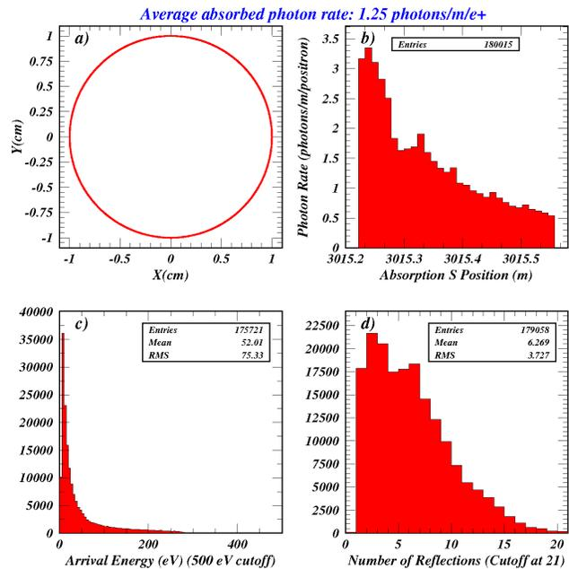
Figure 7: Distributions of absorbed photons in the final-focus quadrupole magnet QC1RP.
