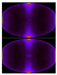
Figure 4: Electron cloud density during the 3rd (top) and 6th (bottom) of 11 time slices during of the passage of bunch 15, which has been offset from the centered bunch train by 1 mm. The "pinched" cloud is centered on the offset bunch. The short bunch length (10 mm) bunch hardly modifies the larger built-up cloud.
