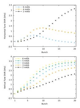
Figure 1: Horizontal (top) and vertical (bottom) tune shift in kHz (to be compared to the revolution frequency of 390 kHz) for a 20 bunch trains of positrons between 2–6 mA/b (3.2– $9.6\times10^{10}$  bunch populations). Data were taken in each plane separately, and only at 2,4, and 6 mA/b in the horizontal plane.
