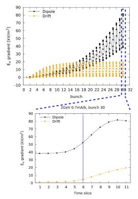
Figure 3: Top: vertical electron cloud space-charge electric field gradients for the 11 time slices within each of 30 bunches, for dipoles and drifts. Bottom: electric field gradients for the 11 time slices in bunch 30, showing the center of the bunch at time slice 6.
