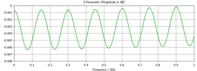
Stripline with tapers to 10 mm electrode on Kapton
