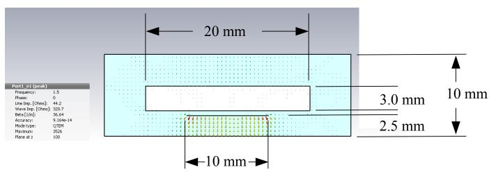
Stripline Simulations: Adding 3 mm thick ceramic results in 15 mm total height and a 3.5 mm collector gap for 50  $\Omega$ .
