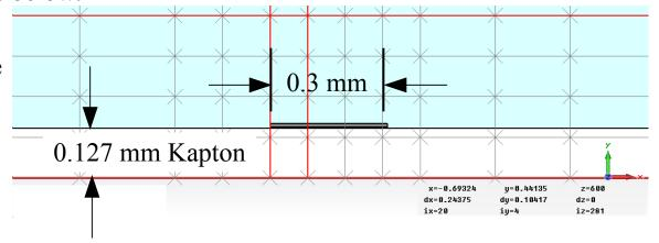
Top view of stripline with tapers to a 10 mm wide electrode on a Kapton substrate
