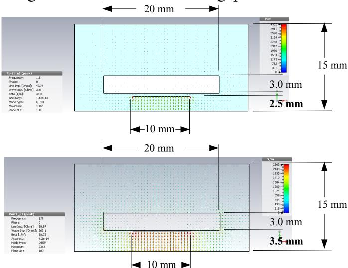
3.5 mm gap with 3 mm ceramic  $50.9 \Omega$
