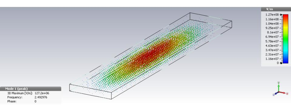
With the ceramic in empty space, the first resonant mode is at 2.5 GHz (3 mm thick, 10 mm wide, 100 mm long)
