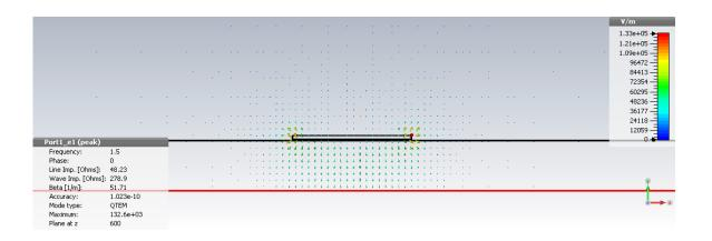
Stripline with tapers to 10 mm electrode on a Kapton substrate
