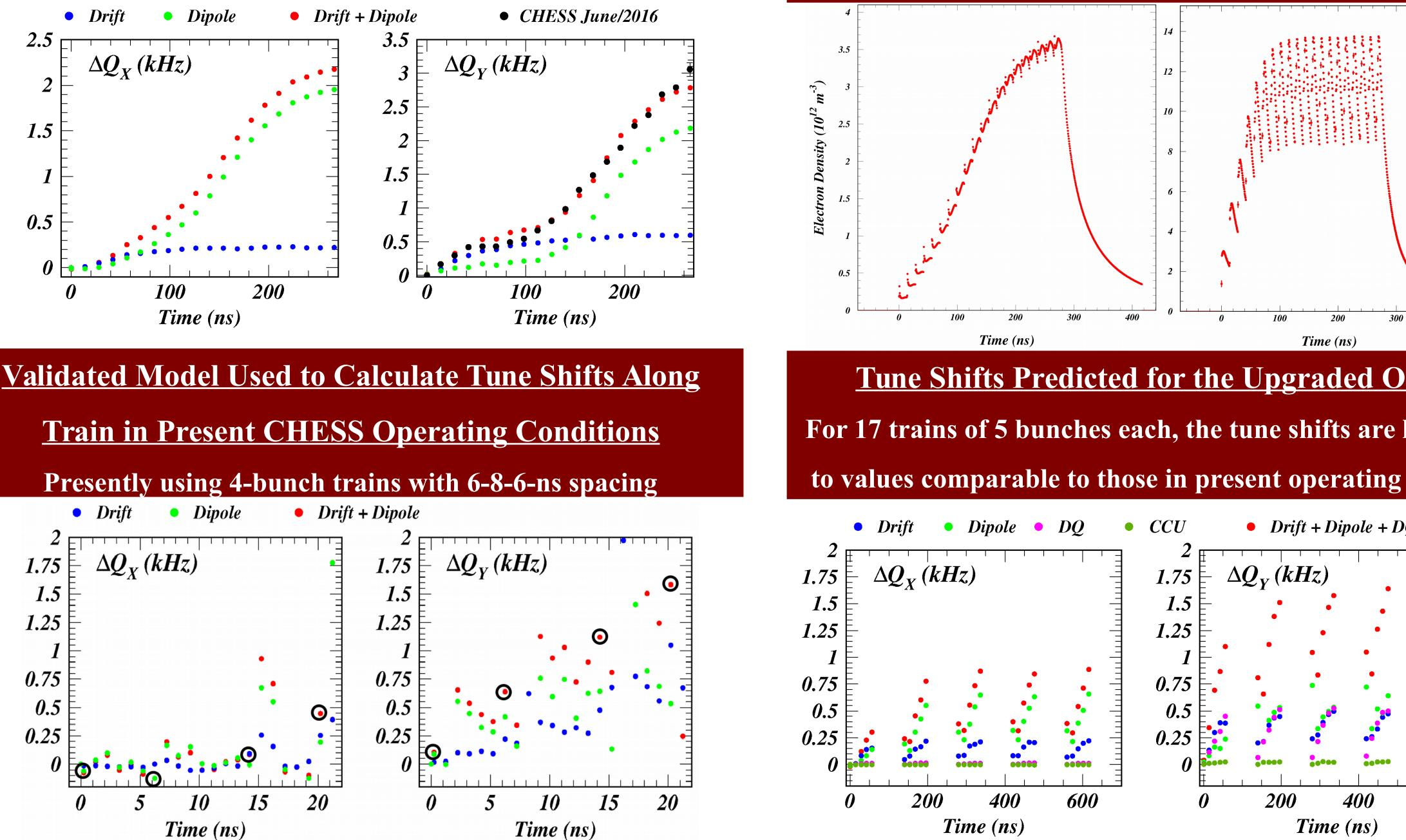
**Comparison of Modeled Electron Cloud Buildup** The cloud density in the c-f magnets is predicted to be a factor of four higher than in the CHESS dipoles now
