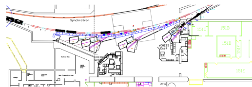
Figure 4: At present CHESS x-ray are generated by counterrotating electron and positron beams. In the proposed reconfiguration x-ray lines are all illuminated by radiation from a single beam traveling counterclockwise. A possible layout of undulator beam lines and accompanying experimental stations in the reconfigured machine are shown.
