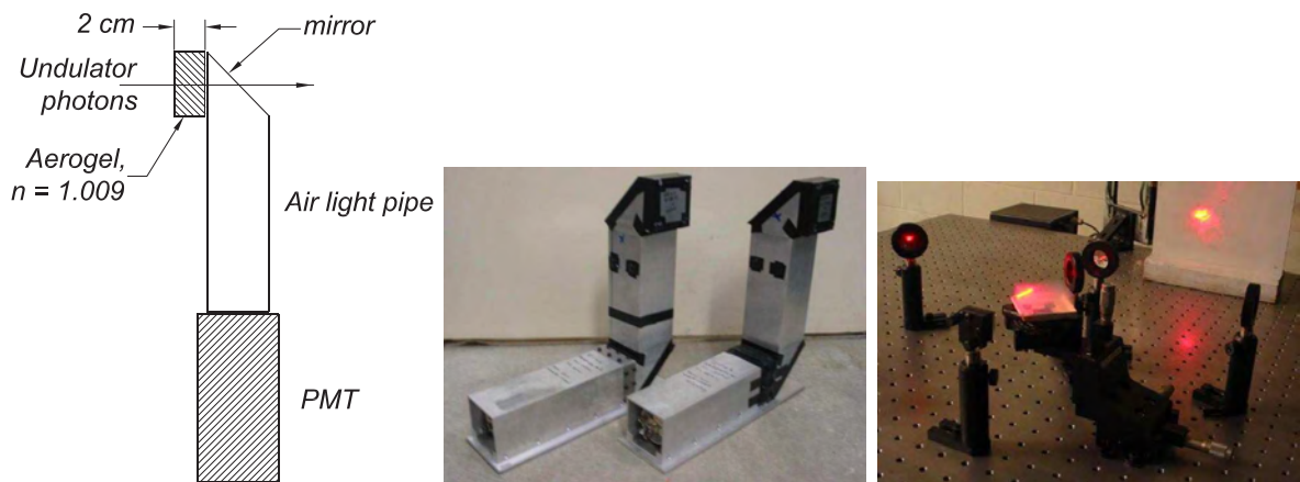
Figure 6: a) Sketch of the photon flux counter, consisting of a 2-cm-thick block of aerogel of index n = 1.009 , viewed by a photomultiplier tube at the end of an air light pipe. b) Photograph of the two aerogel flux counters. c) A block of aerogel mounted in a Michelson interferometer in order to measure its index of refraction [19].
