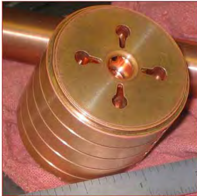
Figure 8. Five-cell NLC accelerating structure used in FY04 investigations.
