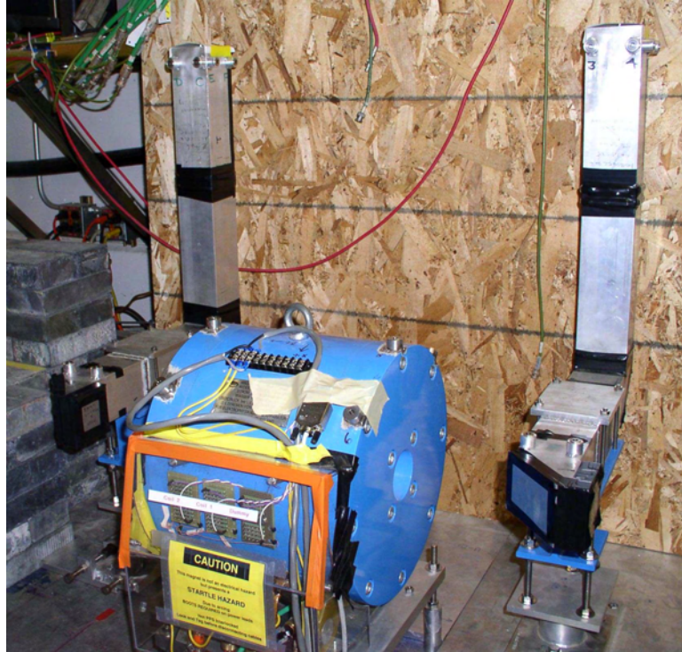
Figure 12: The aerogel detectors in the FFTB tunnel, surrounding the undulator-photon polarimeter solenoid.
