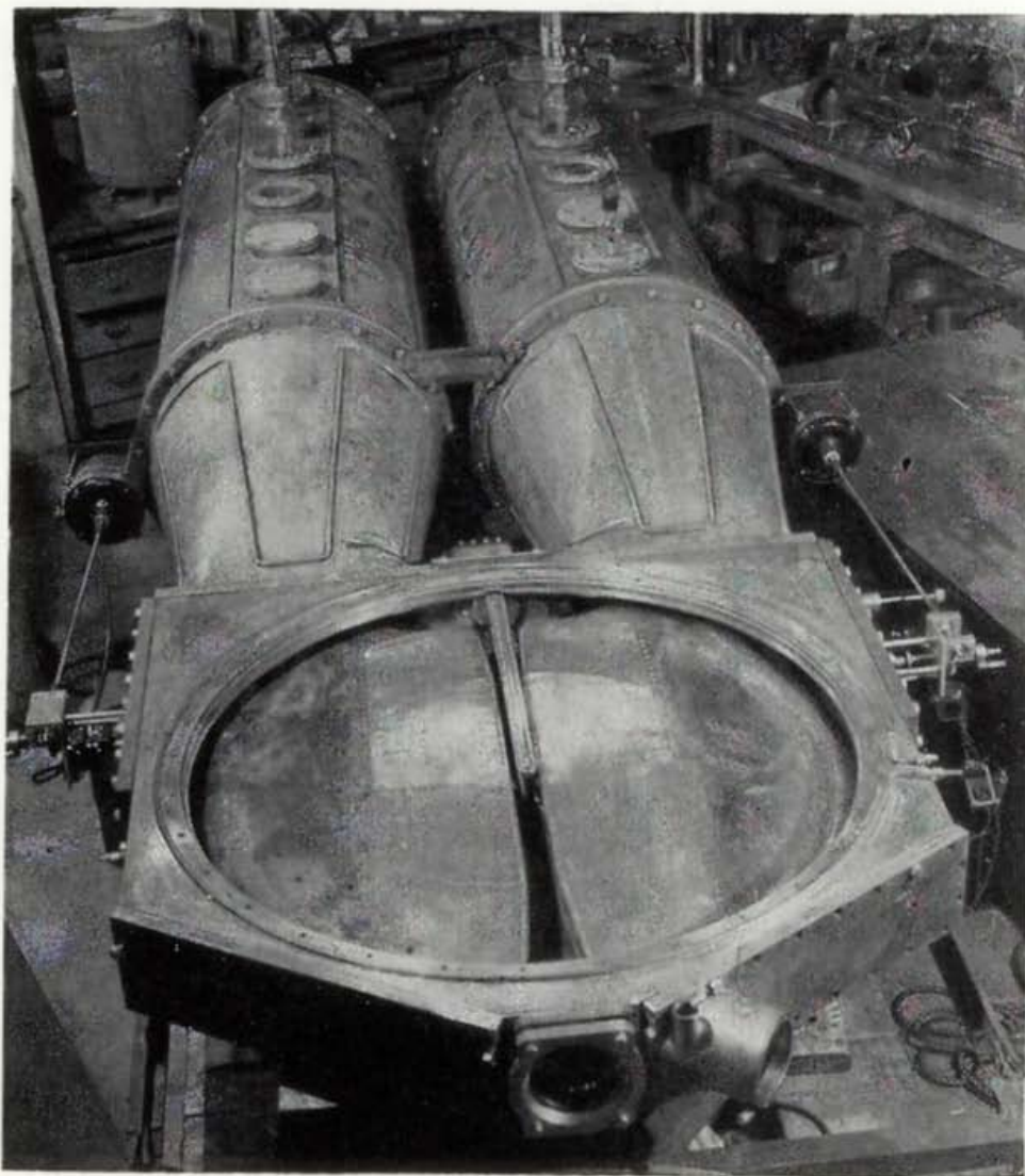
Fig. 6-13. Shop assembly photograph of the MIT cyclotron chamber.
