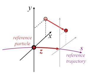
z is approximately the distance along the reference trajectory that a particle is ahead of a reference particle travelling along the reference trajectory with momentum  $P_0$ .
