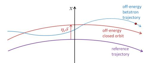
Coupling between transverse and longitudinal planes in a beam line is usually represented by the dispersion,  $\eta_x$ . So, in terms of the horizontal dispersion and betatron action, the horizontal coordinate and momentum of a particle are given by:
