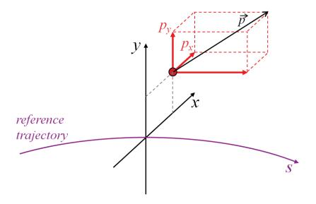
In general, the reference trajectory can be curved. At any point along the reference trajectory, the x and y coordinates are perpendicular to the reference trajectory.
