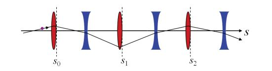
In an uncoupled periodic beam line, particles trace out ellipses in phase space with each pass through a periodic cell.
