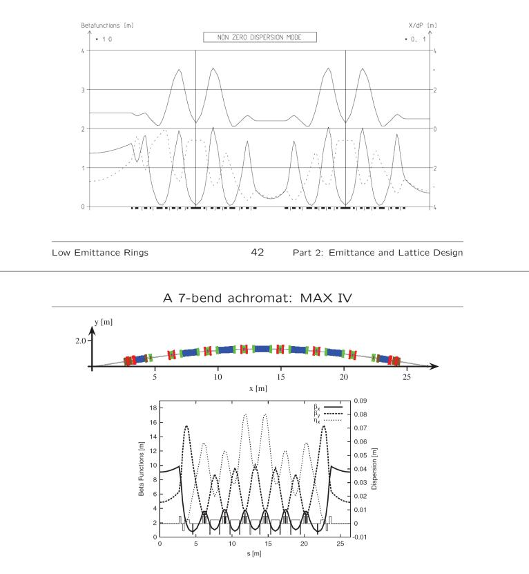
Note: vertical focusing provided by gradient in the bending magnets.
