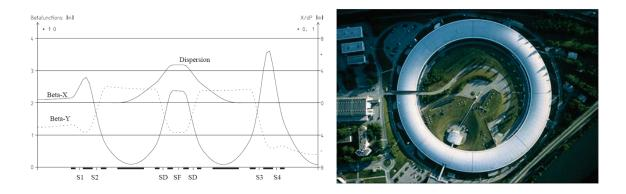
The DBA structure provides a lower natural emittance than a FODO lattice with the same number of dipoles.
