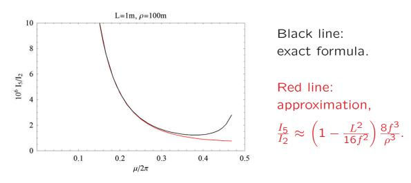
It turns out that the minimum value of the natural emittance in a FODO lattice is given by:
