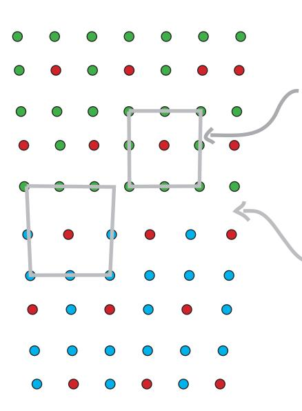
Field wires (in green or blue) form a cage around the sense wire (in red). Sense wires are maintained at 2000V relative to the field wires.
