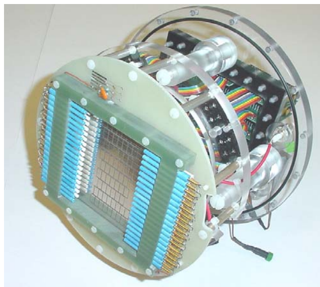
wire gas-amplification stage, readout pads
