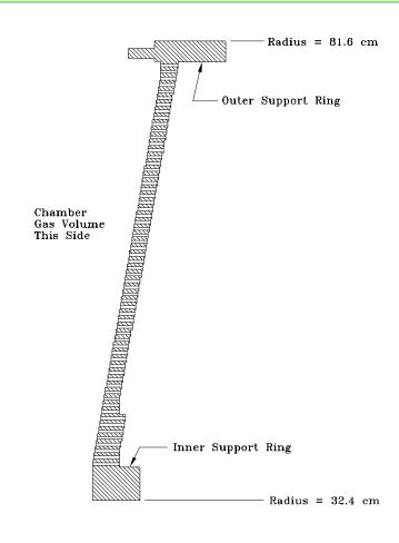
The outer section supports 31 anode layers and associated field wire layers.
