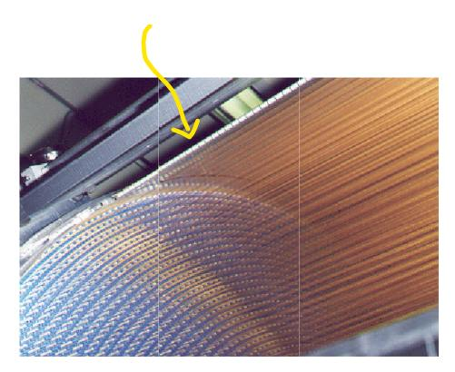
Segmented cathode forms the outer field cage for the outer (47<sup>th</sup>) layer.
