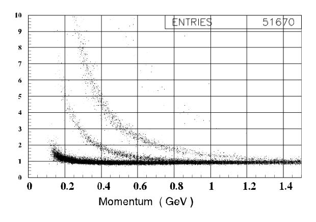
dE/dX measurements for anode measurements
