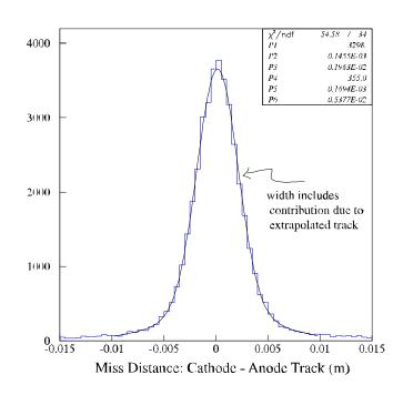
{cathode - "anode track" } resolution includes contribution of extrapolated track ( ~ 1.5 mm)
