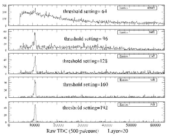
Threshold is set at 0.8  $\mu$ A. with a characteristic time of 8 ns (amplifier rise time), and gas gain ~  $10^5$ , threshold is 0.4 primary ions .
