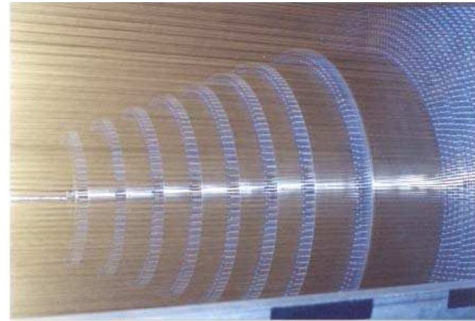
“wedding cake” structure; individual rings and bands The conical “big” plate deforms < 1\text{mm} .
