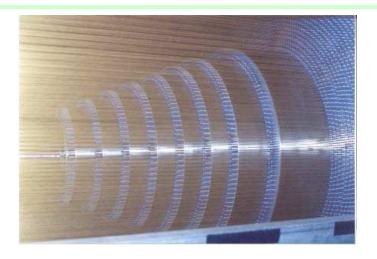
"wedding cake" structure; individual rings and bands The conical "big" plate deforms < 1mm.
