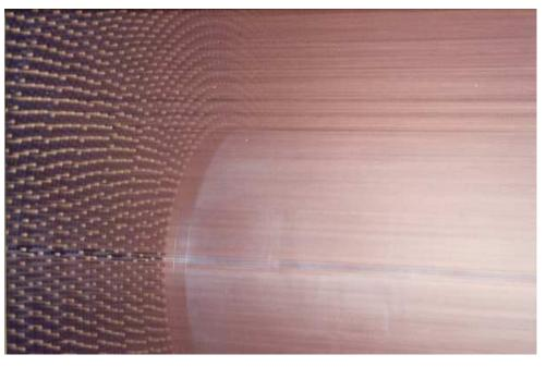
51 layers dense cell design axial superlayers (bushings shown in photo) single stereo layers between the axial superlayers inner and outer cathodes (inner shown in photo) aluminum field wires
