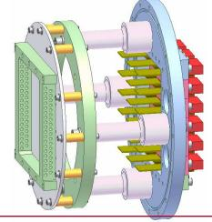
readout end assembly, incl. feedthroughs
