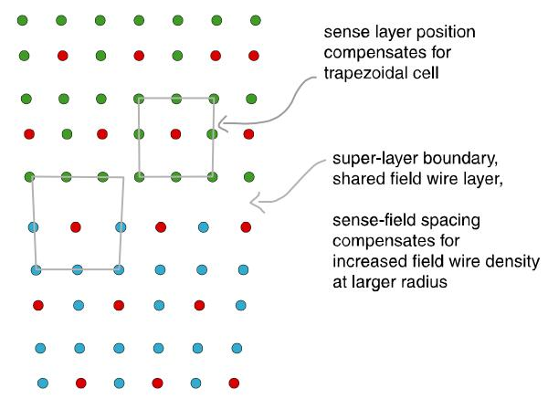
Adjust the sense wire position to compensate for non-uniform field wire density. Drift cells are electrically symmetric in the "r" direction (up-down) direction. Field wire phase is not important.
