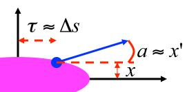
$$\begin{aligned} x' &= \partial_{p_x} K \\ p'_x &= -\partial_x K \end{aligned} \Rightarrow \begin{cases} x' &= \partial_a K/p_0 , \quad a' &= -\partial_x K/p_0 \\ y' &= \partial_b K/p_0 , \quad b' &= -\partial_y K/p_0 \end{cases}$$
