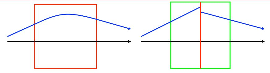
$$\underline{M}_{\text{quad},x}^{\text{thin}}(s) = \begin{pmatrix} 1 & -\frac{s}{2} \\ 0 & 1 \end{pmatrix} \begin{pmatrix} \cos(\sqrt{k}s) & \frac{1}{\sqrt{k}}\sin(\sqrt{k}s) \\ -\sqrt{k}\sin(\sqrt{k}s) & \cos(\sqrt{k}s) \end{pmatrix} \begin{pmatrix} 1 & -\frac{s}{2} \\ 0 & 1 \end{pmatrix} \\
