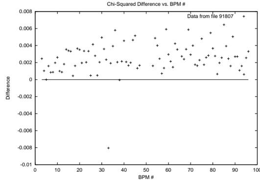
FIG. 4: Plot of difference in  $\chi^2$  fit when the coefficients are not used and when they are. The bpm number is on abscissa. The measurements were taken during one complete orbit in the ring.
