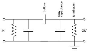
FIG. 2: Beam position monitor circuit diagram.
