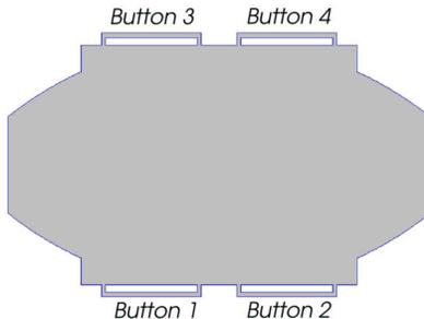
FIG. 1: 2D transverse cross section of Arc BPM used in CESR. The white rectangles represent the buttons and the grey area is the interior of the vacuum pipe.
